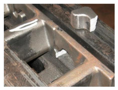
Figure 21. View of one of the damaged toothed segments of the Komtrack system.
