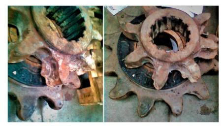
Figure 2. Damaged track wheels of the Eicotrack system.
