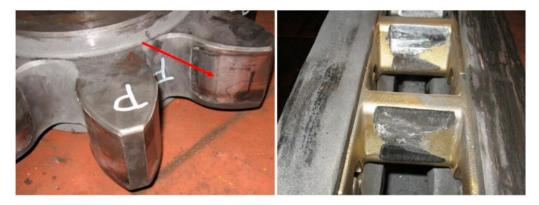
Figure 4. Damages to the track wheel and the Flextrack racks during the field tests.
