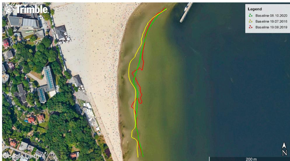
**Figure 5.** The course of the TSB of the waterbody adjacent to the public beach in Gdynia measured with the hydrographic method in 2018–2020.
