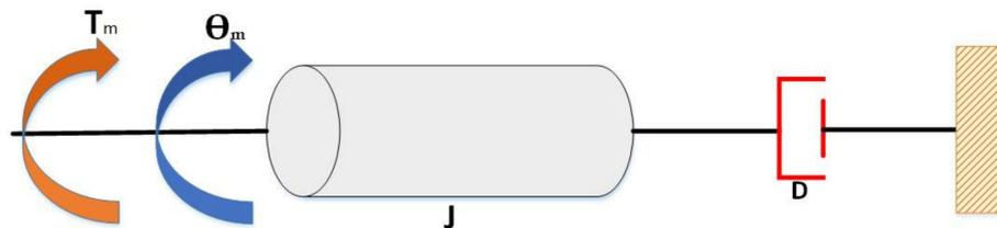
Figure 6. Representation of mechanical load in motor.
