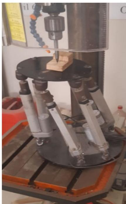
**Figure 16.** Experimental setup. (A pictorial view of the test being carried out by machining bed on a workpiece).
