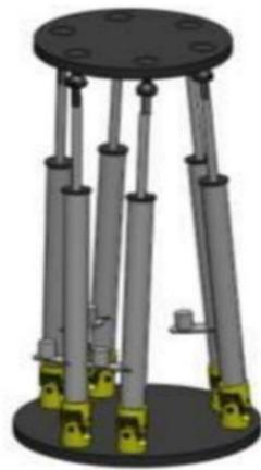
Figure 2. SolidWorks<sup>(R)</sup> model of the proposed Machining Bed.
