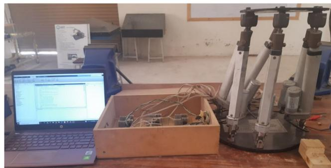
**Figure 14.** Fabricated model of the six DOF machining bed.
