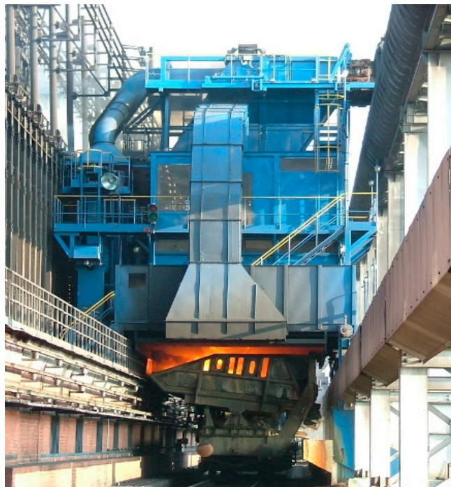
Figure 3. Dedusting system on the coke side. Source: Instytut Chemicznej Przeróbki Węgla (IChPW; Institute for Chemical Processing of Coal) materials from the implementation of the project 'Intelligent coking plant meeting the requirements of the best available technology'.
