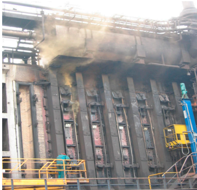
Figure 2. Fugitive emission from leaks in the coke battery door. Source: Instytut Chemicznej Przeróbki Węgla (IChPW; Institute for Chemical Processing of Coal) materials from the implementation of the project 'Intelligent coking plant meeting the requirements of the best available technology'.
