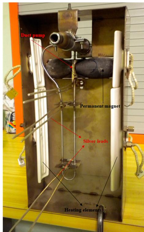
Figure 1. Picture of the current resistivity meter.
