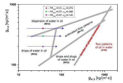
**Figure 12.** Selected series of simulations for  $\eta_r = 100$  vs. two-phase liquid–liquid flow structures.
