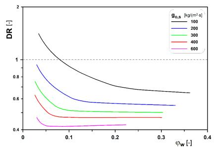
**Figure 5.** Variations in the *DR* index for oil with a viscosity of  $\eta_r = 100$ .
