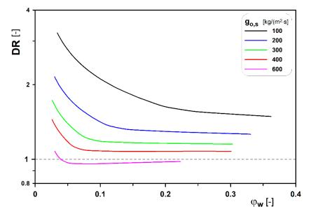
**Figure 7.** Variations in *DR* index for oil with the viscosity of  $\eta_r = 25$ .
