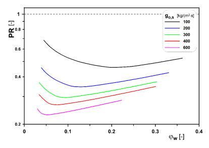
**Figure 10.** Variations in *PR* index for oil with the viscosity  $\eta_r = 300$ .
