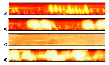
**Figure 2.** Selected two-phase liquid–liquid flow structures in a tube with a diameter of 12 mm (photos from the author's archive) (**a**) water droplets in oil, (**b**) plugs and drops of water in oil, (**c**) water dispersion in oil,(**d**) film-dispersed flow of phases.
