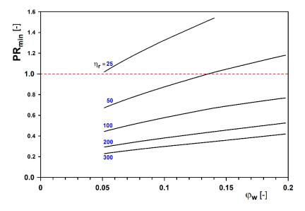
Figure 11. Smallest viable values of PR for oils with various viscosities.
