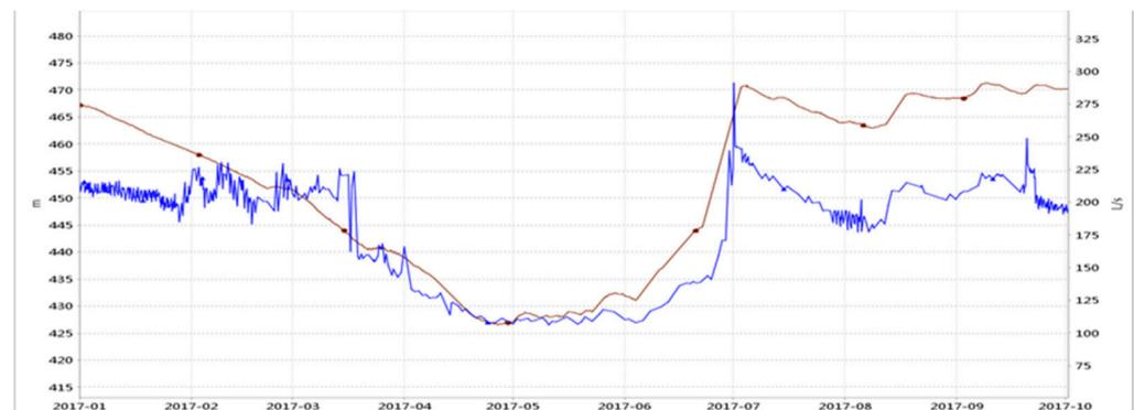
**Figure 7.** Statistical data for the upstream water level (red line) and the seepage discharge (blue line).
