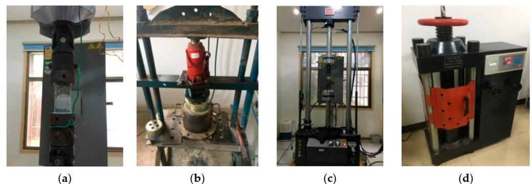
**Figure 2.** Overall photo of test setup: (a) deformability; (b) impermeability; (c) bond strength; (d) compressive strength tests.
