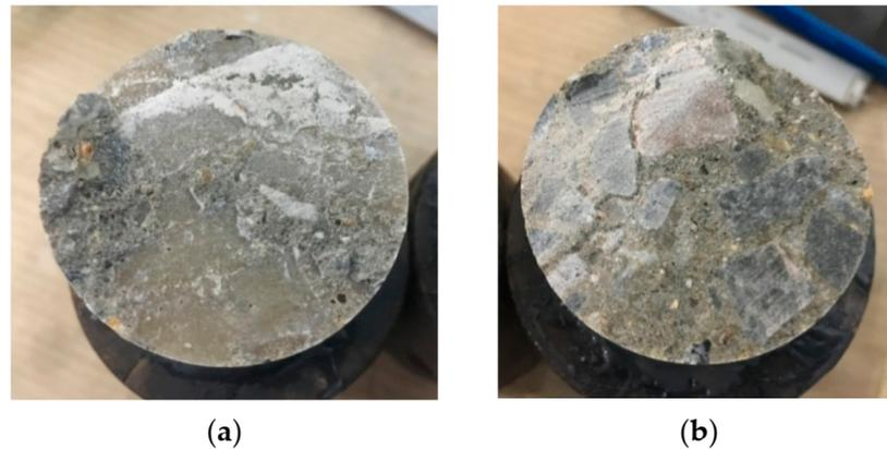
**Figure 3.** Debonding failures of the sample of F1 without cracks (a) lower end-face; (b) upper end-face.
