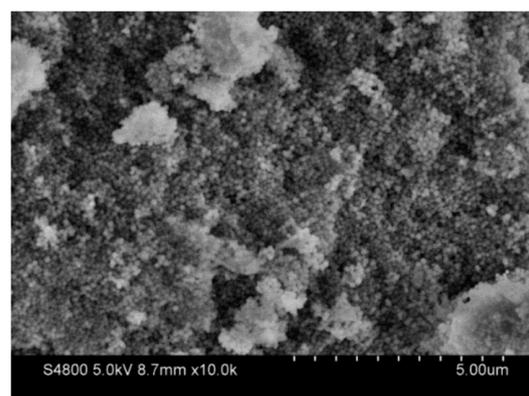
**Figure 4.** The SEM image of the SN-modified underwater composite-repairing material.
