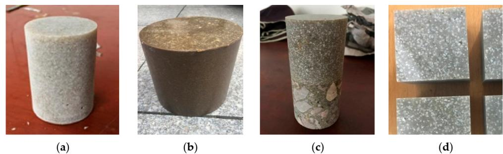
**Figure 1.** Test specimens of the SN-modified underwater composite-repairing material: (a) deformability; (b) impermeability; (c) bond strength; (d) compressive strength tests.
