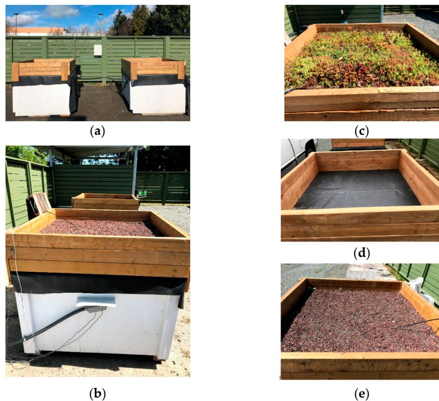
**Figure 2.** (a) Two experimental test cells; (b) cables routing from inside; (c) green roof test cell surface (d) bare roof test cell surface; (e) roof with 150 mm thick substrate test cell surface.
