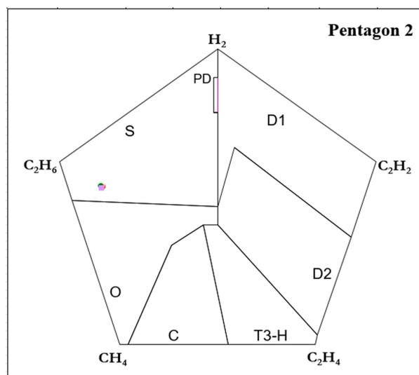
**Figure 4.** SG patterns of DDB oil in bushings of RWE in service (units 3–4).
