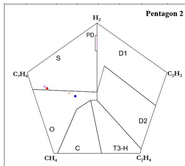
**Figure 2.** SG patterns of DDB oil during SG tests at 120 °C and 200 °C in the laboratory.
