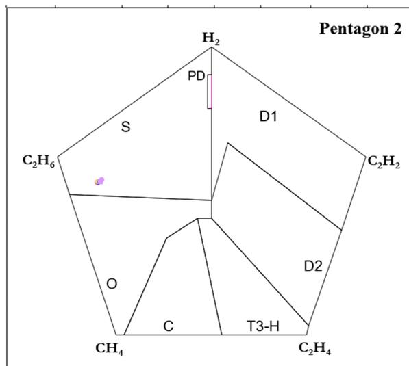
**Figure 3.** SG patterns of DDB oil in bushings of RWE in service (units 1–2).
