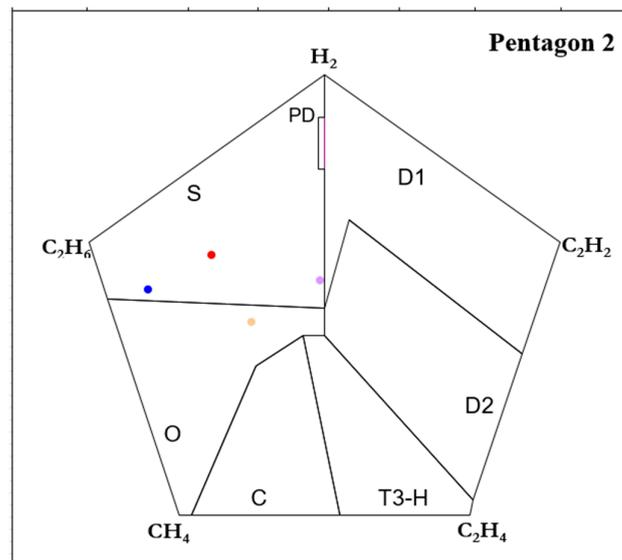
**Figure 5.** SG patterns of DDB oil during SG tests at 80 °C to 200 °C in the laboratory.
