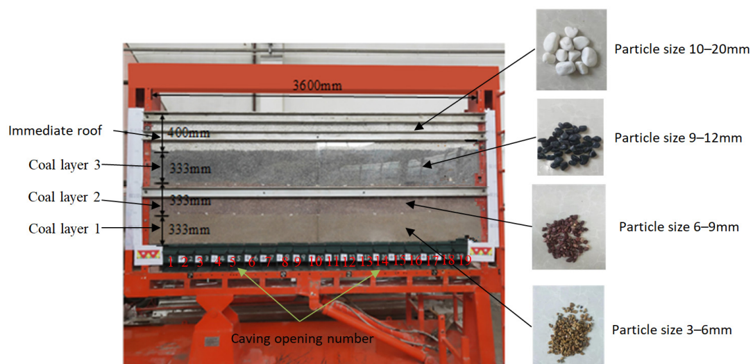
Figure 10. Physical picture of laying scheme.
