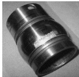
**Figure 26.** Defect in the inner ring of bearing 3.
