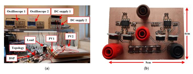
Figure 11. Photograph showing: (a) Complete experimental setup, (b) Designed prototype.
