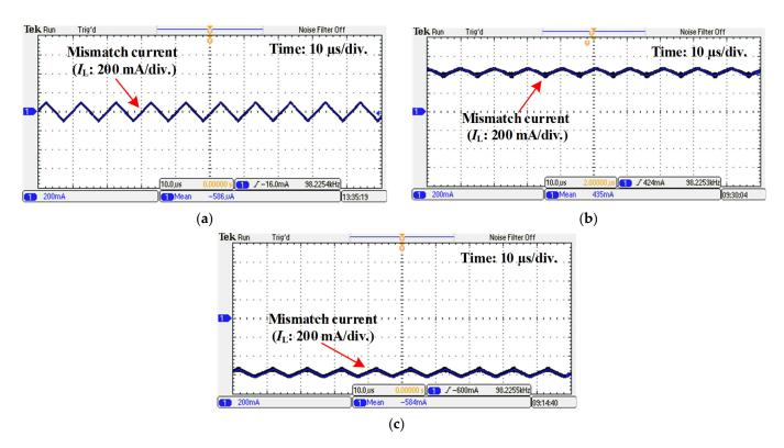
**Figure 12.** Experimental results showing mismatch current ( $I_L$ ) for various test conditions in Table 5 for *SCL*-based *DPP* topology. (a) Test 1 (b) Test 2 and (c) Test 3.
