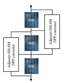
Figure 3. General structure of submodule-to-submodule (SM-SM) mismatch mitigation DPP converter.
