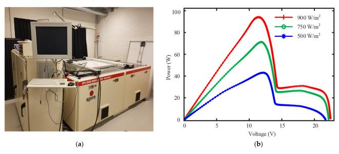
**Figure 4.** Experimental evaluation of the mismatch effect on a solar PV module (Solvis: SV36-150) containing three submodules with bypass diodes: (a) SPI-SUN 5600 SLP solar sun simulator, (b) Power-voltage (P-V) characteristics when one of the PV cells is shaded from the three submodules and overall irradiance levels are 900 W/m², 750 W/m², and 500 W/m².
