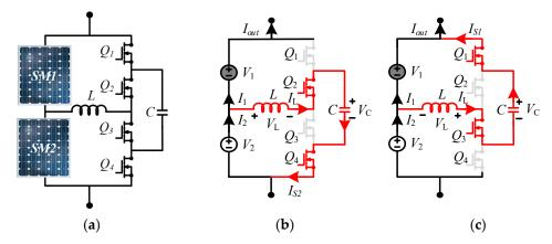
**Figure 5.** Proposed DPP topology (a) General circuit, (b) Energizing state/mode 1: power flow when SM2 is producing more than SM1, (c) De-energizing state/mode 2: power flow when SM2 is producing more than SM1. Here, L and C are switched-inductor and switched-capacitor used for the mismatch energy processing.  $I_{S1}$  and  $I_{S2}$  are the currents flowing through the switches  $Q_1$ ,  $Q_2$ ,  $Q_3$ , and  $Q_4$ .
