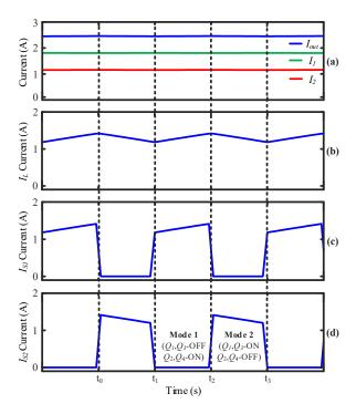
**Figure 8.** Simulated results under scenario 2 (SM1 is shaded) for the proposed SCL-based DPP topology: (a) Output current and submodules current, (b) mismatch current ( $I_L$ ) passing through the inductor L (c) current passing through  $Q_1$  and  $Q_3$ , (d) current passing through  $Q_2$  and  $Q_4$ .
