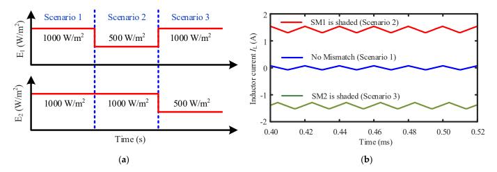
**Figure 7.** Mismatch scenarios and results: (**a**) Mismatch scenarios (scenario 1: when SM1 and SM2 is producing Scheme 2. when SM1 producing lower than SM2, and scenario 3: when SM2 is producing lower than SM1), (**b**) Mismatch current ( $I_L$ ) passing through the inductor L under various mismatch scenarios in Figure 7a.
