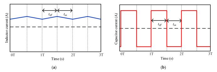
**Figure 6.** Basic operational waveforms during mismatch: (a) Current flowing through the inductor *L*, (b) Current flowing through the capacitor *C*, where *T* is the switching period.
