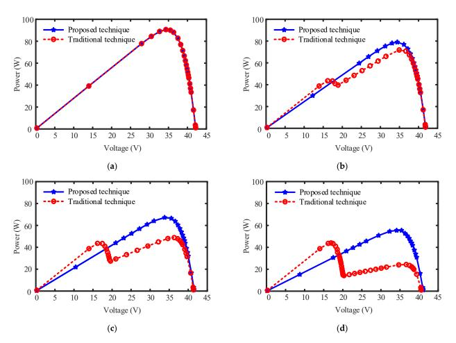
**Figure 9.** *P-V* characteristics for the proposed topology under mismatch cases given in Table 2 for proposed *DPP* and traditional bypass diode technique (a) Case 1, (b) Case 2, (c) Case 3, (d) Case 4.
