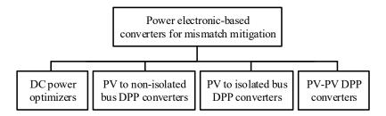
Figure 2. Power electronic-based mismatch mitigation solutions.
