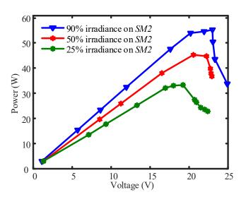
**Figure 13.** Experimentally achieved *P-V* characteristics for the proposed technique when *SM2* in Figure 5 is producing 90%, 50%, and 25% of *SM1* (30 W).
