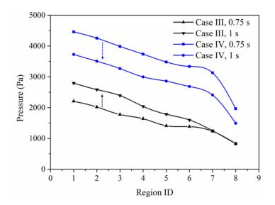
**Figure 12.** Average pressure distribution along the flow direction in case III (alternate injection) and case IV (alternate injection).
