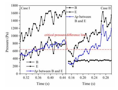
**Figure 7.** Variation of water phase pressure near the oil–water interface with time when oil–water interface starts to move in case I (continuous injection) and case II (continuous injection) (square-line: water pressure near interface B; circle-line: water pressure near interface E; star-line: water pressure difference between B and E).
