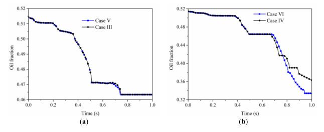
**Figure 21.** Comparison of oil saturation variation with time between slug injection and alternate injection: (**a**) small particles, (**b**) large particles.
