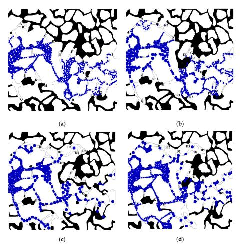
**Figure 10.** Particle–oil–water distribution at different times in case III (alternate injection) and case IV (alternate injection). (a) Case III at 0.75 s; (b) case III at 1 s; (c) case IV at 0.75 s; (d) case IV at 1 s.
