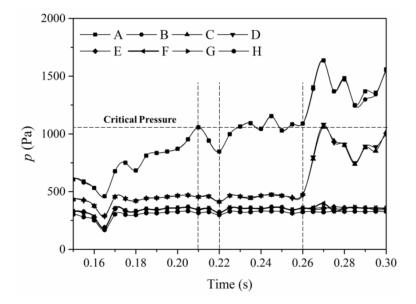
**Figure 5.** Change of the pressure in the water side of water–oil interface when remaining oil starts to move in case II (continuous injection).
