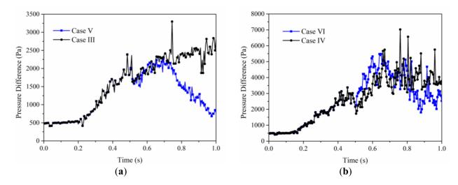
**Figure 20.** Comparison of pressure difference between slug injection and alternate injection with time: (**a**) small particles, (**b**) large particles.
