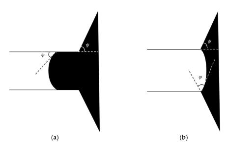
**Figure 3.** The interface morphology when the oil–water interface is in different positions: (**a**) the oil–water interface is in the throat; (**b**) the oil–water interface is in the pore throat interface.
