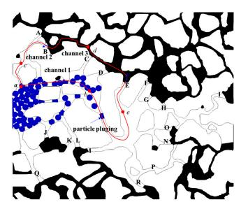
**Figure 4.** Distribution of particle–water–oil in the porous media at 0.26 s when remaining oil starts to move in case II (continuous injection).
