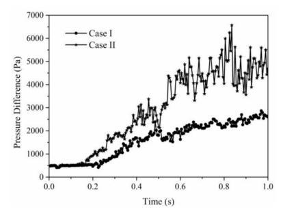
**Figure 8.** Variation of pressure difference between inlet and outlet with time during continuous injection of large or small particles.
