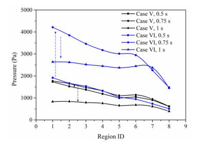
**Figure 15.** Average pressure distribution along the flow direction in case V (slug injection) and case VI (slug injection).
