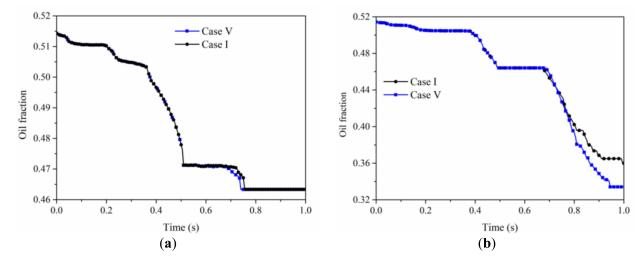
Figure 17. Oil saturation variation with time in continuous injection and slug injection (a) small particles (b) large particles.
