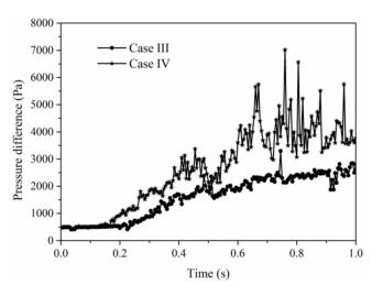
**Figure 11.** Variation of inlet–outlet pressure difference with time in case III (alternate injection) and case IV (alternate injection).
