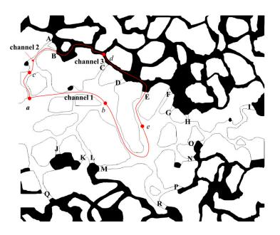
Figure 2. Oil and water two-phase distribution (black represents oil, white represents water).
