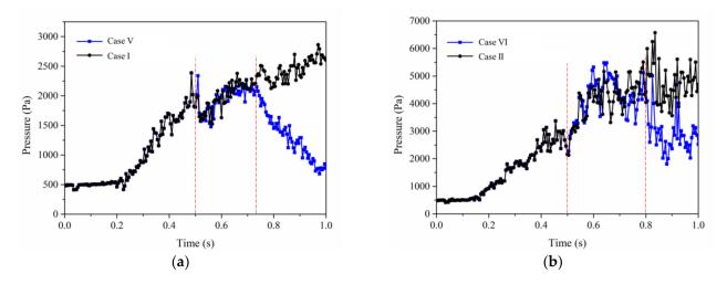
**Figure 16.** Comparison of inlet–outlet pressure difference variation with time between continuous injection and slug injection: (**a**) small particles, (**b**) large particles.
