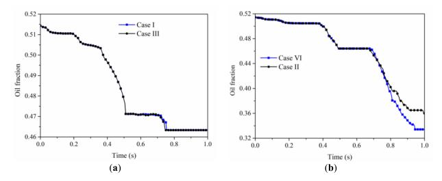
**Figure 19.** Comparison of oil saturation variation with time between continuous injection and alternate injection: (**a**) small particles, (**b**) large particles.
