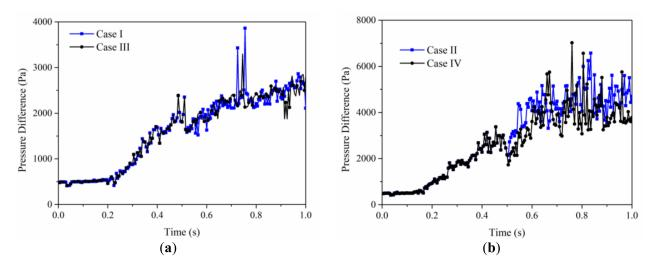
**Figure 18.** Comparison of inlet–outlet pressure difference with time between continuous injection and slug injection: (**a**) small particles, (**b**) large particles.
