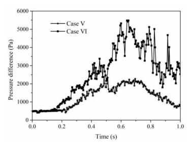
**Figure 14.** Variation of inlet–outlet pressure difference with time in cases V (slug injection) and VI (slug injection).
