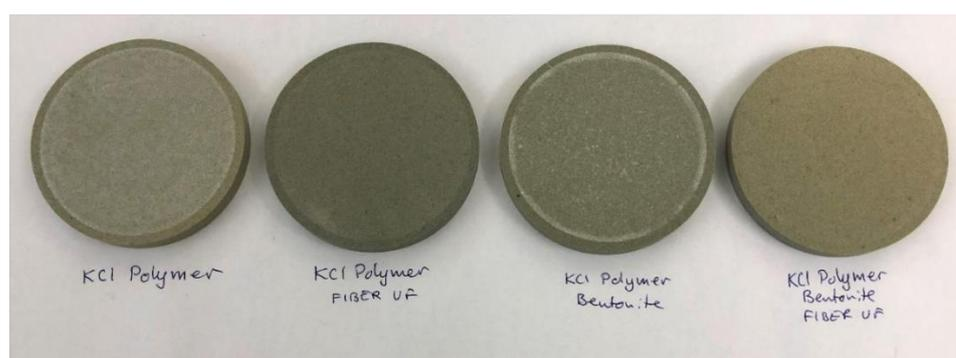
**Figure 9.** Discs from tests 12–15 after breaker application and drying.
