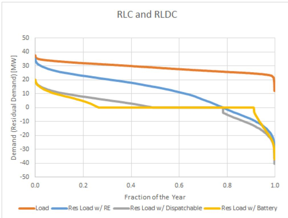
Figure S14 - Load duration curve (orange) and residual load duration curves (RLDCs) considering variable renewable energy (VRE) only (blue), VRE + dispatchable renewable (gray) and including battery storage (yellow)
