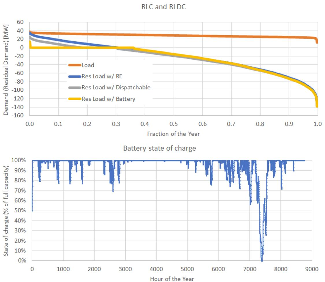
Figure S15 - (Top) RLDC as in the previous figure, but for a system with relatively low dispatchable renewable energy capacity; demand is satisfied for very nearly all hours. (Bottom) Battery state of charge throughout the year is such that the system is usually fully charged; a large battery capacity is necessary in the absence of dispatchable power capacity, although that full battery capacity is needed for only very few hours of the year.
