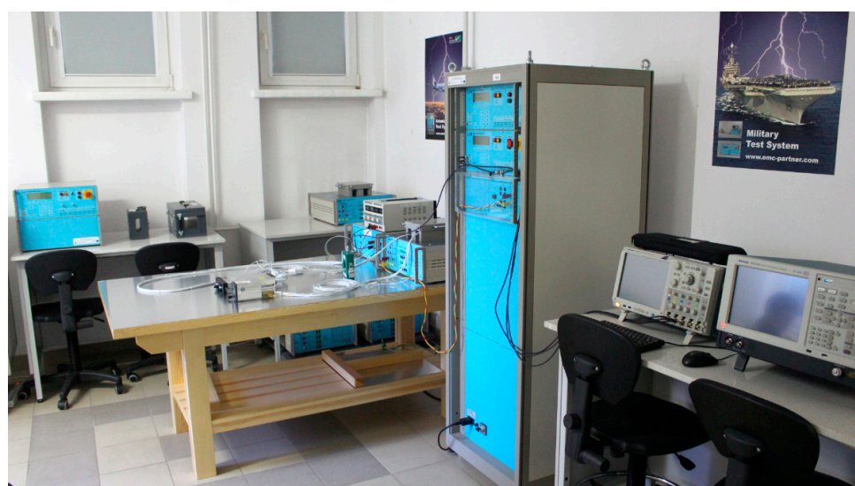
Figure 5. General view of the test stand dedicated to indirect lightning tests of avionics immunity.
