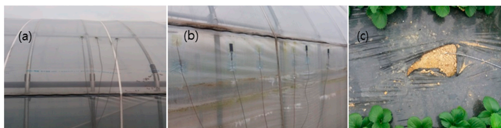
Figure 2. Photographs of the greenhouse with the heat flow sensors: (a) roof, (b) side, and (c) floor.
