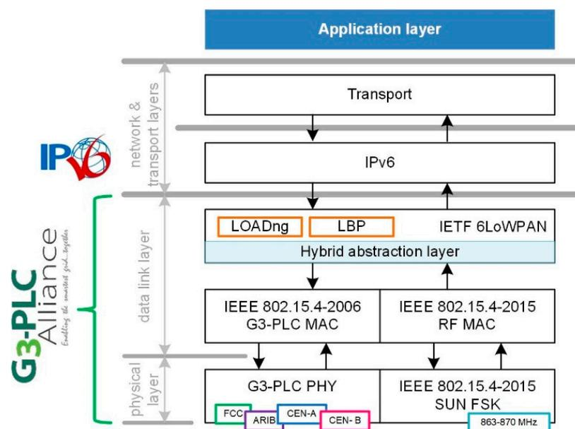
Figure 14. The G3-PLC Hybrid PLC & RF protocol stack.
