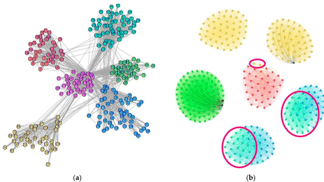
**Figure 8.** Telecom communities mapped over the G3-PLC network topology (a) and over existing cartographic data related to the network’s electrical topology (b).
