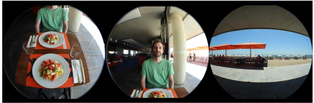
**Figure 2.** Real pictures of Sal Café restaurant with each workplane: table, a person in front and window. For each picture, the High Dynamic Range (HDR) of three exposures,  $-2$ ,  $0$  and  $2$ , has been obtained and they are ISO 400 and  $8.0 \text{ M } 3456 \times 2304$  image quality (Canon EOS 600D, with Canon objective EFS 18–55 mm).
