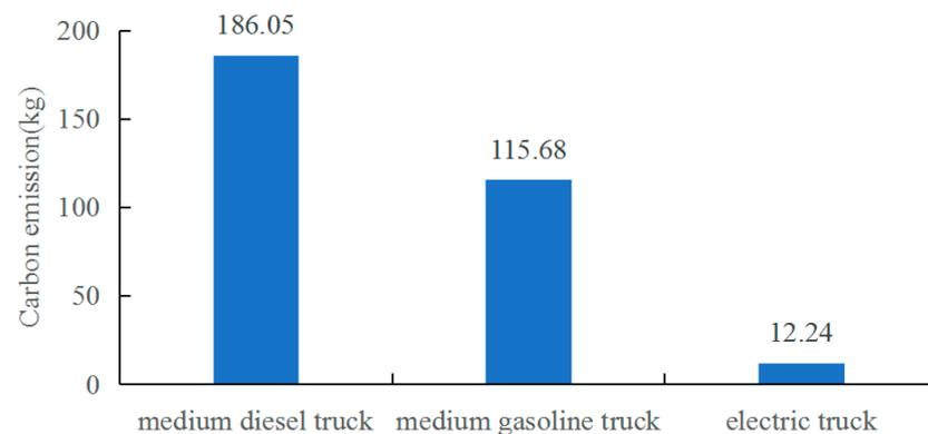
**Figure 9.** Carbon emissions from CG-2 composite beams transported by different energy vehicles.
