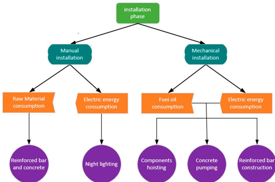
Figure 4. Carbon emissions sources of prefabricated components during the installation stage.
