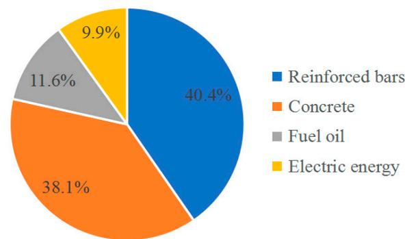
**Figure 8.** Proportion of carbon emissions generated by various materials and energy consumption of CG-2 composite beams during the production stage.
