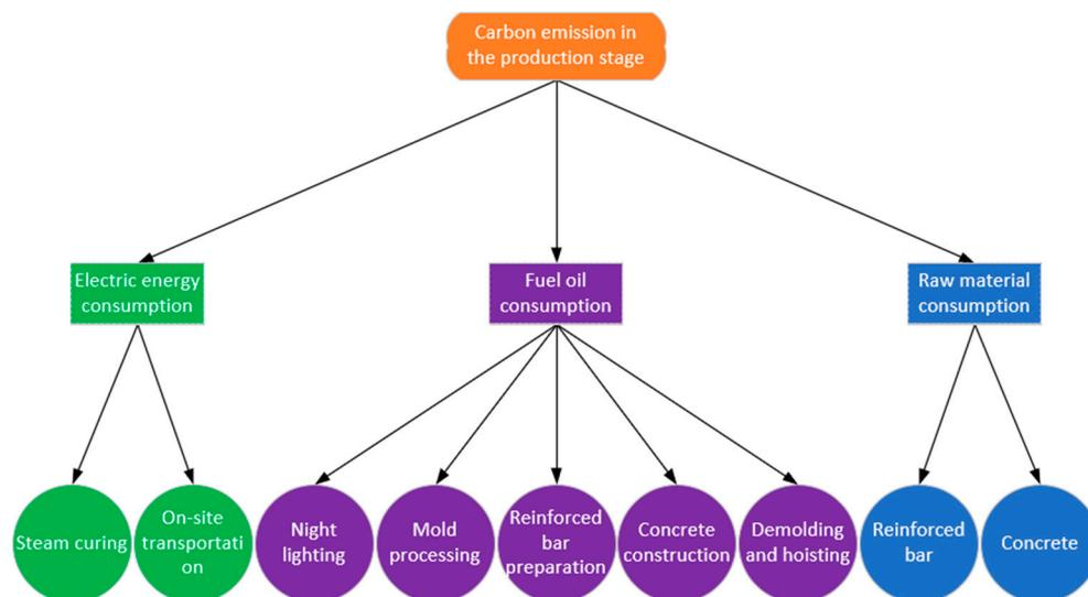
**Figure 2.** Carbon emissions sources of prefabricated components during the production stage.
