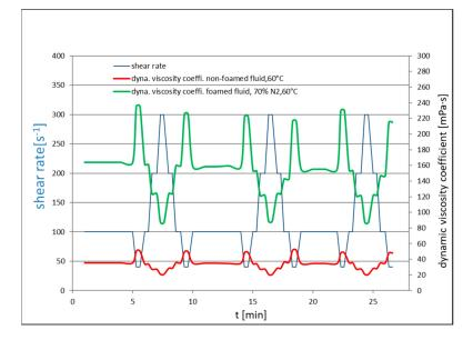
Figure 4. Viscosity of non-foamed FF1A and N<sub>2</sub>-foamed FF1B fluid of 70% quality at 60  $^{\circ}$ C.
