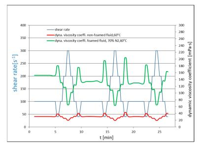
Figure 5. Viscosity of non-foamed FF2A and N<sub>2</sub>-foamed FF2B fluid of 70% quality at 60  $^\circ$ C.
