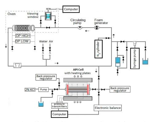
Figure 3. The simplified diagram of the measurement unit for testing the fracture conductivity and damaging it by foamed fracturing fluids.
