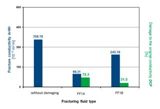
**Figure 6.** The damage to the primary conductivity of the fracture filled with quartz sand proppant 20/40 done by fracturing fluids FF1A and FF1B at a temperature of 60 °C; compressing stress 27.6 MPa.
