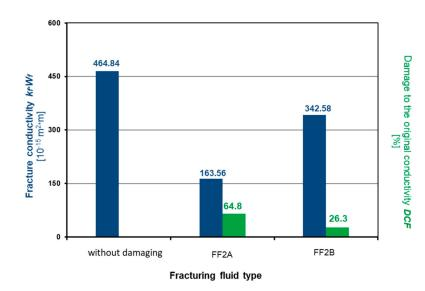
**Figure 7.** The damage to the primary conductivity of the fracture filled with light ceramic proppant 20/40 done by fracturing fluids FF2A and FF2B at a temperature of 60 °C; compressing stress 41.4 MPa.
