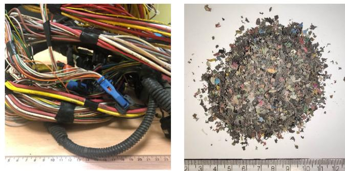
**Figure 2.** Automotive shredder residue (ASR) plastic sample before and after the grinding process.
