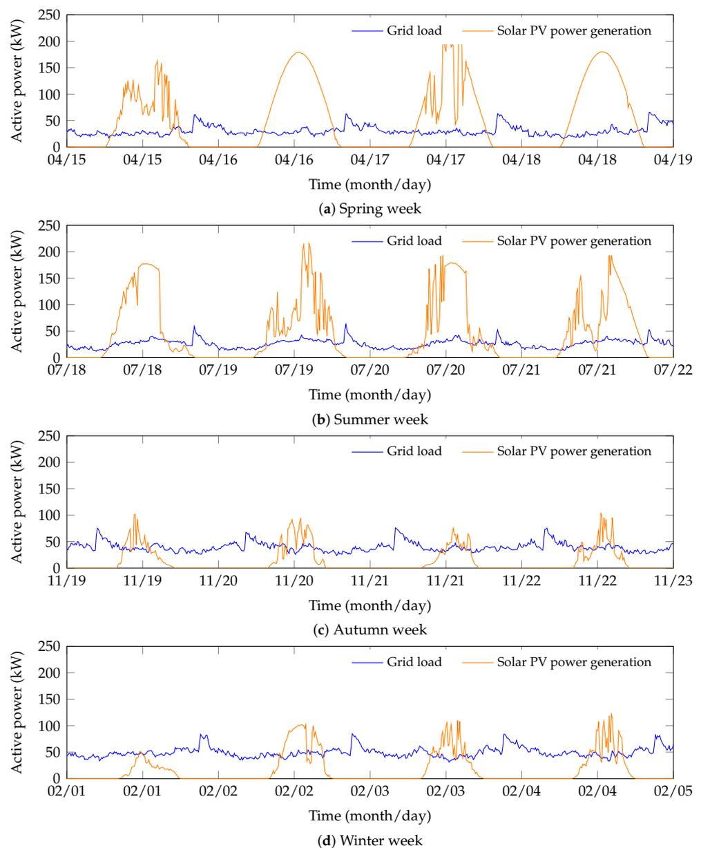
**Figure 1.** The grid load (transformer-level measurements of power consumption in a suburban neighbourhood composed of approximately 120 households) and solar PV power generation (50 household PV panels) over four “season-typical” weeks: a spring week (a); a summer week (b); an autumn week (c); and a winter week (d).
