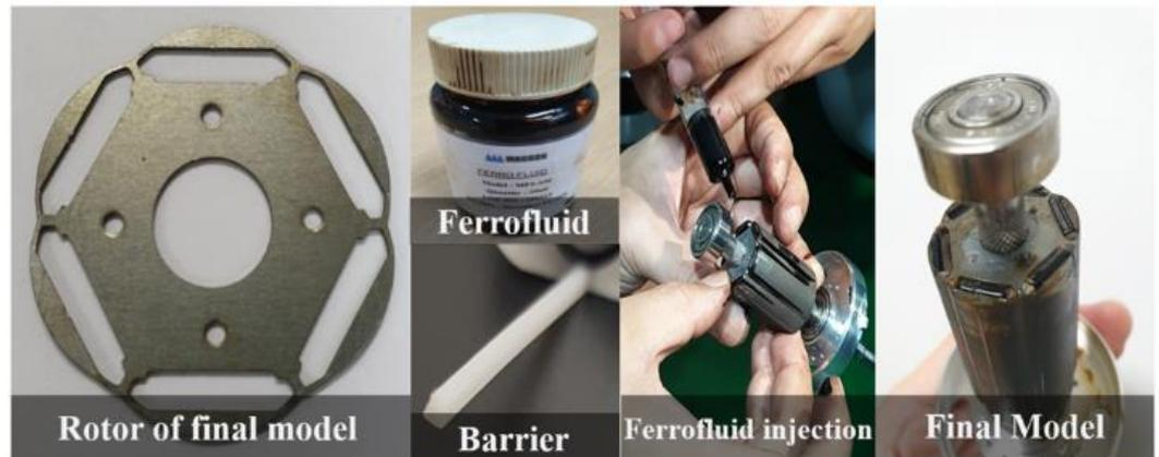
Figure 21. Process of setting up the experimental equipment.
