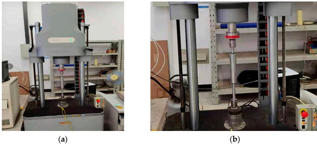
**Figure 3.** Damping characteristics test of the magnetorheological fluid damper. (a) Instron E10000 electronic dynamic testing machine; (b) MRF damper installed on the dynamic testing machine.
