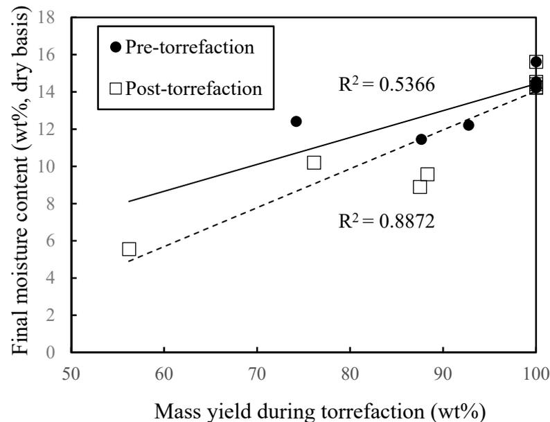
**Figure 3.** Relationship between the mass yield during torrefaction and the final moisture content of the pellets at 85% RH. Mass yield of 100% refers to normal pellets.
