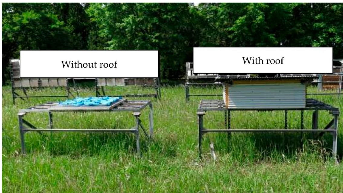
Figure 1. Overview of outdoor weathering test.
