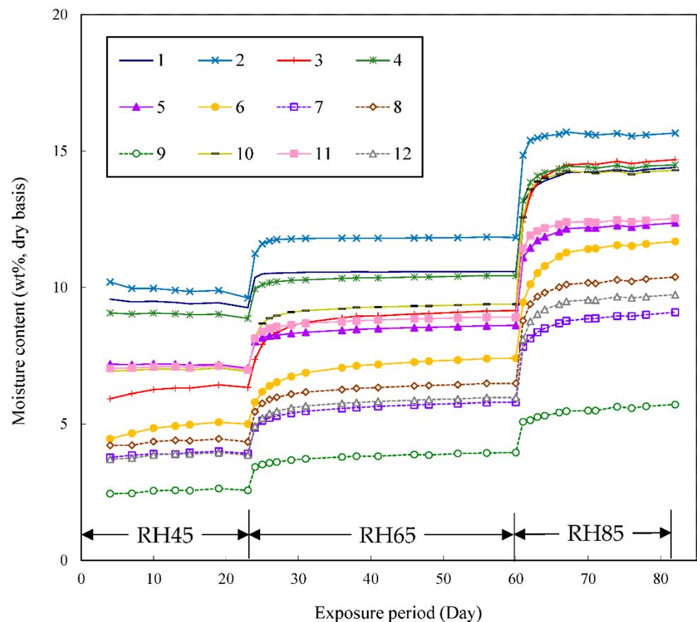
**Figure 2.** Changes in the moisture content of each pellet type during exposure to three stages of relative humidity (RH) conditions. Each item in the legend corresponds to a pellet sample number shown in Table 1. Solid, open, and the other symbols represent pre-torrefied, post-torrefied, and normal pellets, respectively.
