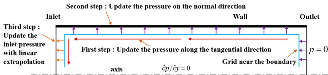
Figure 4. Schematic diagram of pressure boundary treatment in circular tube.
