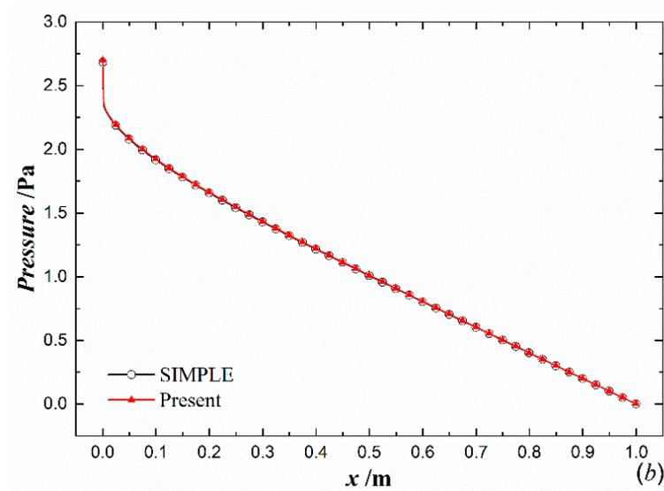
Figure 5. Fluid velocity along central line (a) and boundary pressure on tube wall (b).
