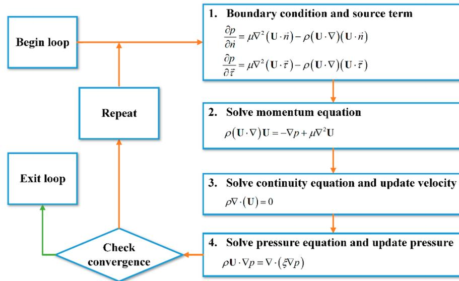
Figure 2. Flow chart for pressure-velocity coupling method.
