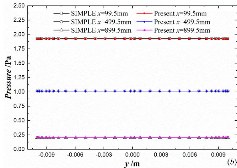
Figure 7. Velocity (a) and pressure (b) at the cross section of tube.
