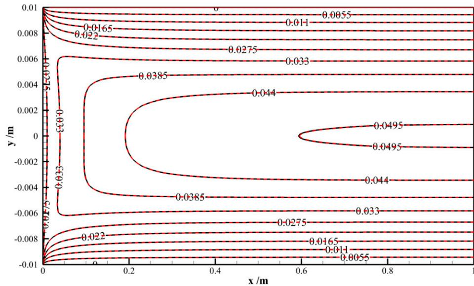
**Figure 8.** The comparison of velocity magnitude contours in the tube-axis plane, m/s.
