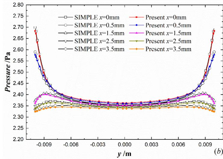
Figure 6. Fluid velocity (a) and pressure (b) at the cross section of entrance region.
