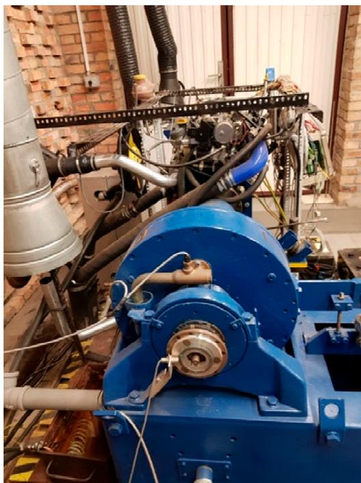
**Figure 1.** The test stand for the Fiat 1.3 JTD (Jet Turbo Diesel) engine at Wrocław University of Science and Technology.**Table 2.** Selected physicochemical properties of the tested fuels.
