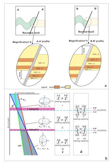
**Figure 9.** (a). The Shale Gouge Ratio (SGR) value of AA' section is equal to that of BB' section. In AA' and BB' sections, the dip angle and strike of faults are the same, and the stratigraphic characteristics are also the same. (b) The AA' and BB' sections are under different stress regimes. (c) The depth and stress regimes of AA' and BB' are the same. (d) The depths of AA' and BB' are different, and the stress regimes are also different.
