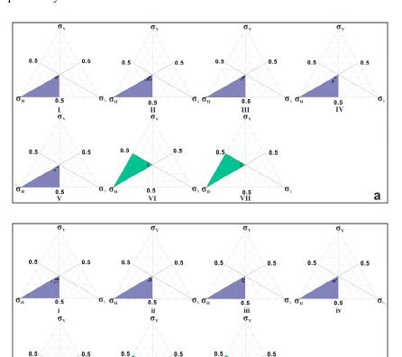
**Figure 7.** Ternary diagrams showing the stress state near the fault plane of F3 (**a**) and F4 (**b**) (see Figure 5c for detailed settings). The blue shade represents the reverse fault regime, whereas the green shade represents the strike slip regime.
