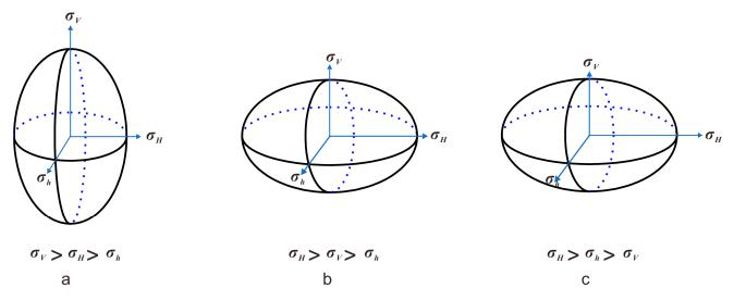
**Figure 2.** Present in situ stress state of the fault plane; (a) Normal fault stress regime (NF); (b) Strike-slip fault regime (SS); (c) Reverse fault stress regime (RF).
