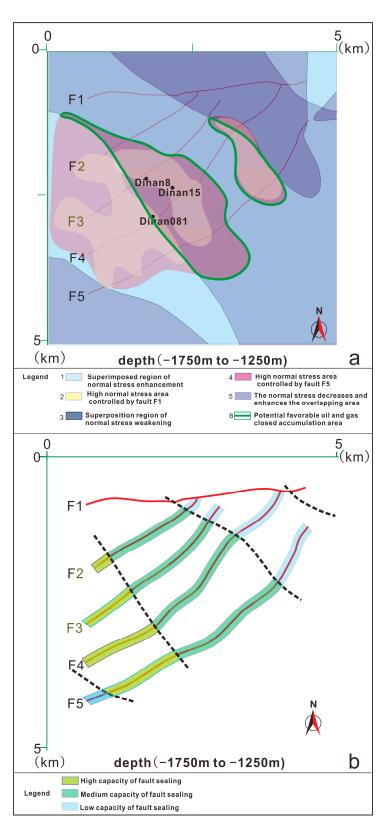
**Figure 11.** (a) Superposition analysis chart of numerical simulation based on normal stress change of the fault plane. (b) Schematic diagram of classification and evaluation of fault sealing based on normal stress intensity of fault plane.
