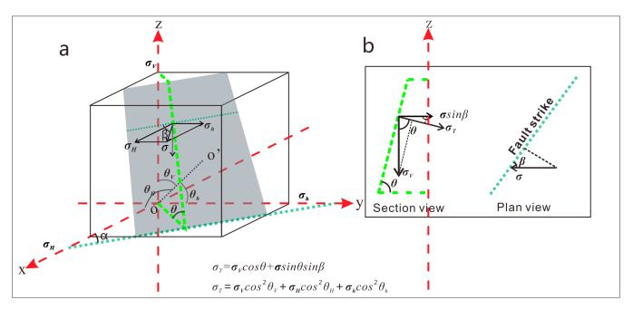
**Figure 3.** Schematic diagram of depth conversion of fault zone and stress state regime of cross-section. (oo' is the normal of the fault plane;  $\theta_V$ ,  $\theta_H$  and  $\theta_h$  are the angles between  $\sigma_V$ ,  $\sigma_H$ ,  $\sigma_h$  and the normal out of the fault plane, respectively). (a) A description of the stress on the fault plane from a space view. (b) A description of the stress on the fault plane from a sectional view.
