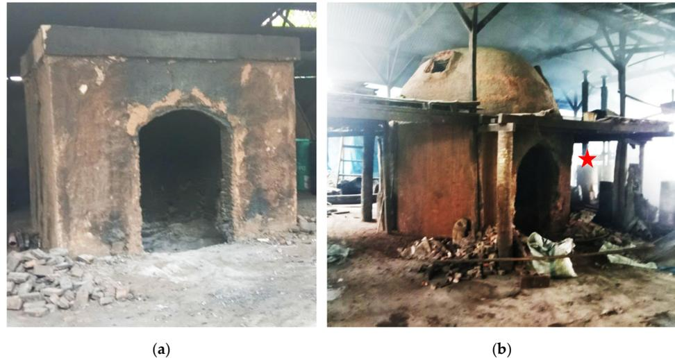
**Figure 1.** (a) Box furnace and (b) dome furnace. The red star symbol at (b) is the condenser system.
