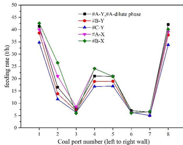
Figure 8. Fuel distributions during the measurement of at different ports.
