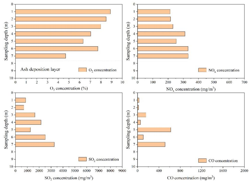
Figure 7. Vertical distributions of flue gas composition at the #B SNCR inlet.
