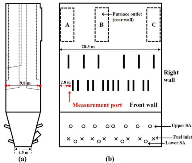
**Figure 3.** Positions of the horizontal measurement ports in the dilute phase: (a) view from the side wall; and (b) view from the front wall.
