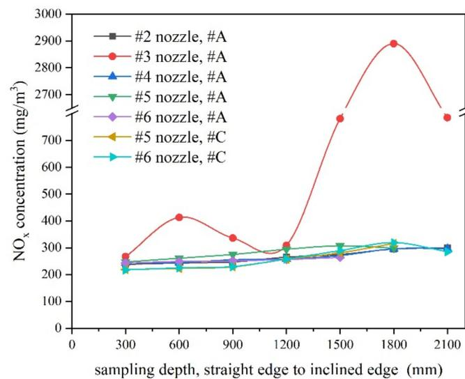
**Figure 10.** Horizontal distributions of  $\text{NO}_x$  concentration at the different heights of the #A and #C SNCR inlets.
