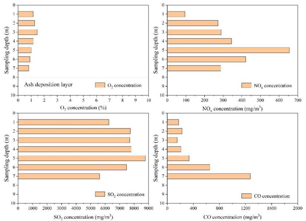
**Figure 9.** Vertical distributions of flue gas composition at the #C SNCR inlet.
