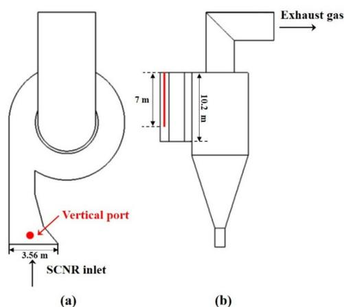
**Figure 2.** Positions of the vertical measurement ports of the three SNCR inlets: (a) top view; and (b) side view.
