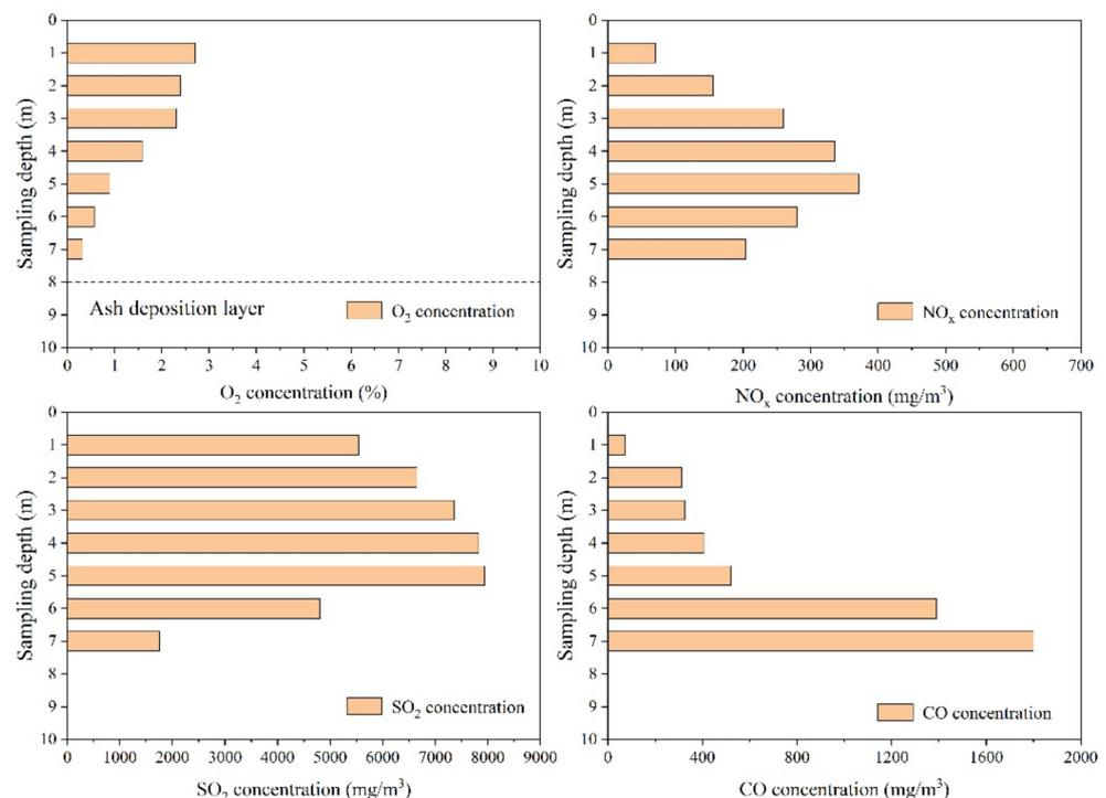
**Figure 5.** Vertical distributions of flue gas composition at the #A SNCR inlet.
