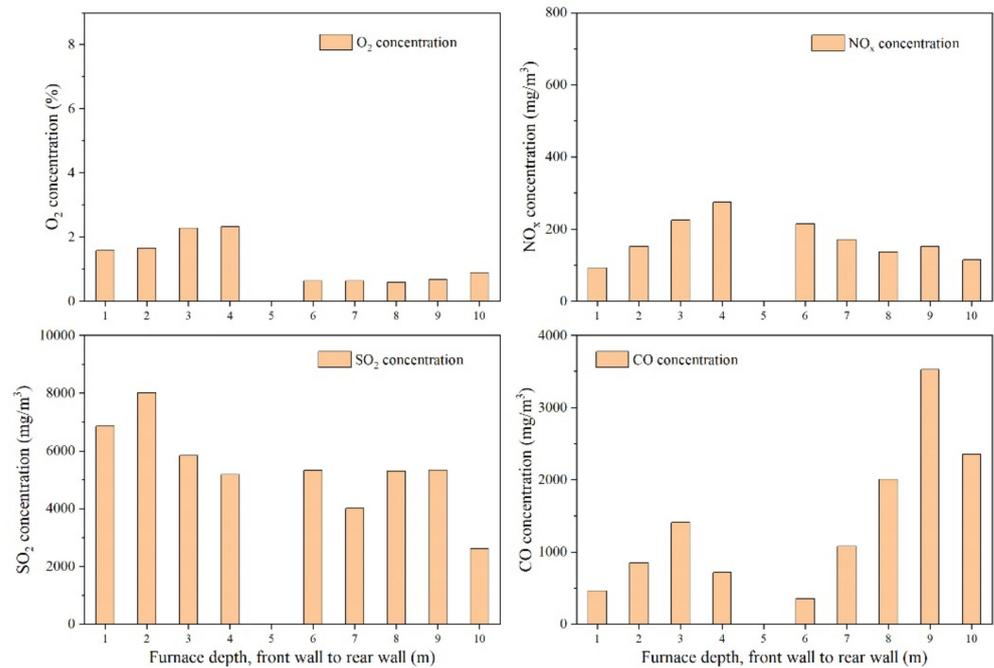
**Figure 6.** Horizontal distributions of flue gas composition at the dilute phase zone corresponding to the #A SNCR inlet.
