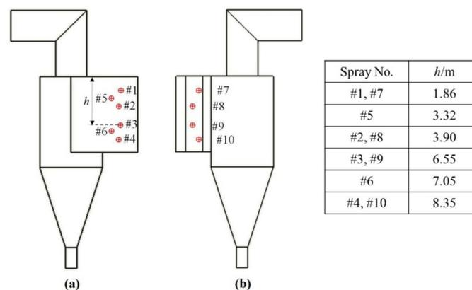
**Figure 4.** Detailed positions of the urea pray guns/horizontal measurement ports at SNCR inlets: (a) view from the straight edge; and (b) view from the inclined edge.
