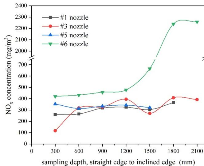
**Figure 11.** Horizontal distributions of NO<sub>x</sub> concentration at the different heights of the #B SNCR inlet.
