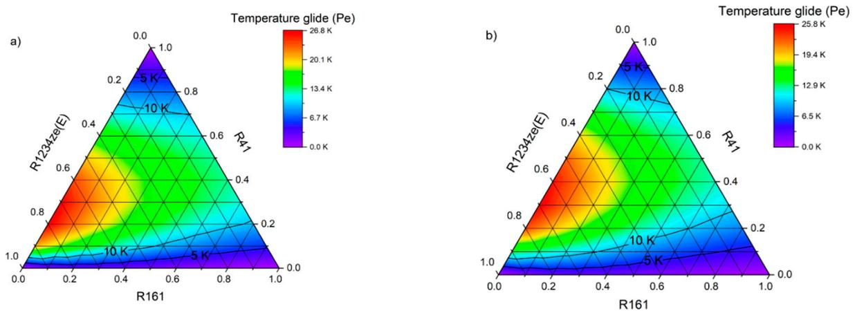
**Figure 8.** Temperature glide at the evaporation pressure for cooling cycles with R161–R41–R1234ze(E) mixture as refrigerant: (a) AC system ( $t_e/t_c = 0/30$  °C); (b) low-temperature system ( $t_e/t_c = -30/30$  °C).
