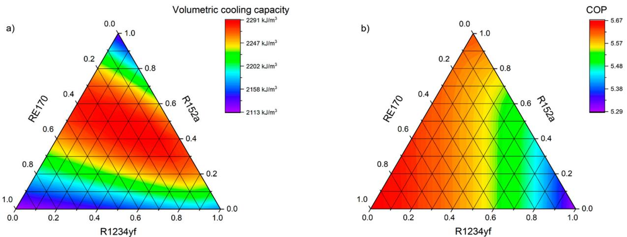
**Figure 13.** Volumetric cooling capacity (a) and (b) the COP for air-conditioning system ( $t_e/t_c = 0/30\text{ }^\circ\text{C}$ ) with R1234yf–R152a–RE170 mixture as refrigerant.
