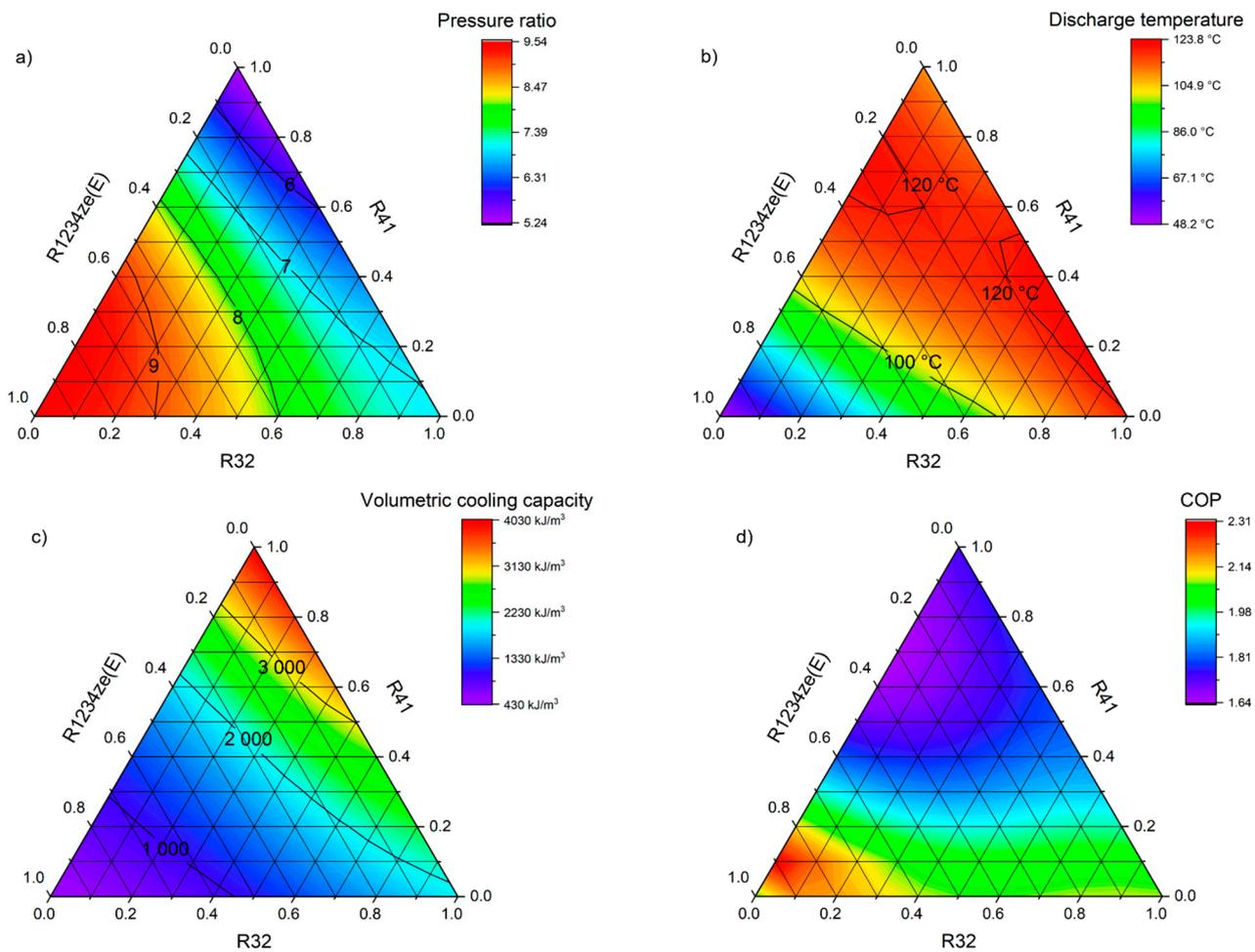
**Figure 6.** Low-temperature system parameters ( $t_e/t_c = -30/30\text{ °C}$ ) of the R32–R41–R1234ze(E) mixture: (a) pressure ratio; (b) temperature of the refrigerant vapour at the compressor discharge; (c) volumetric cooling capacity; and (d) COP.
