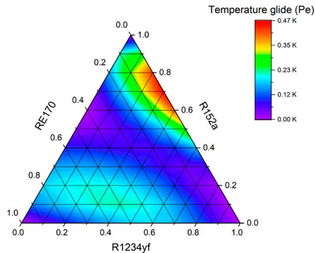
**Figure 12.** Temperature glide at the evaporation pressure for air-conditioning system ( $t_e/t_c = 0/30\text{ }^\circ\text{C}$ ) with R1234yf–R152a–RE170 mixture as refrigerant.
