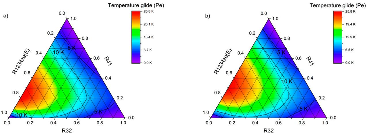
**Figure 4.** Temperature glide at the evaporation pressure for cooling cycles with R32–R41–R1234ze(E) mixture as refrigerant: (a) AC system ( $t_e/t_c = 0/30$  °C); (b) low-temperature system ( $t_e/t_c = -30/30$  °C).
