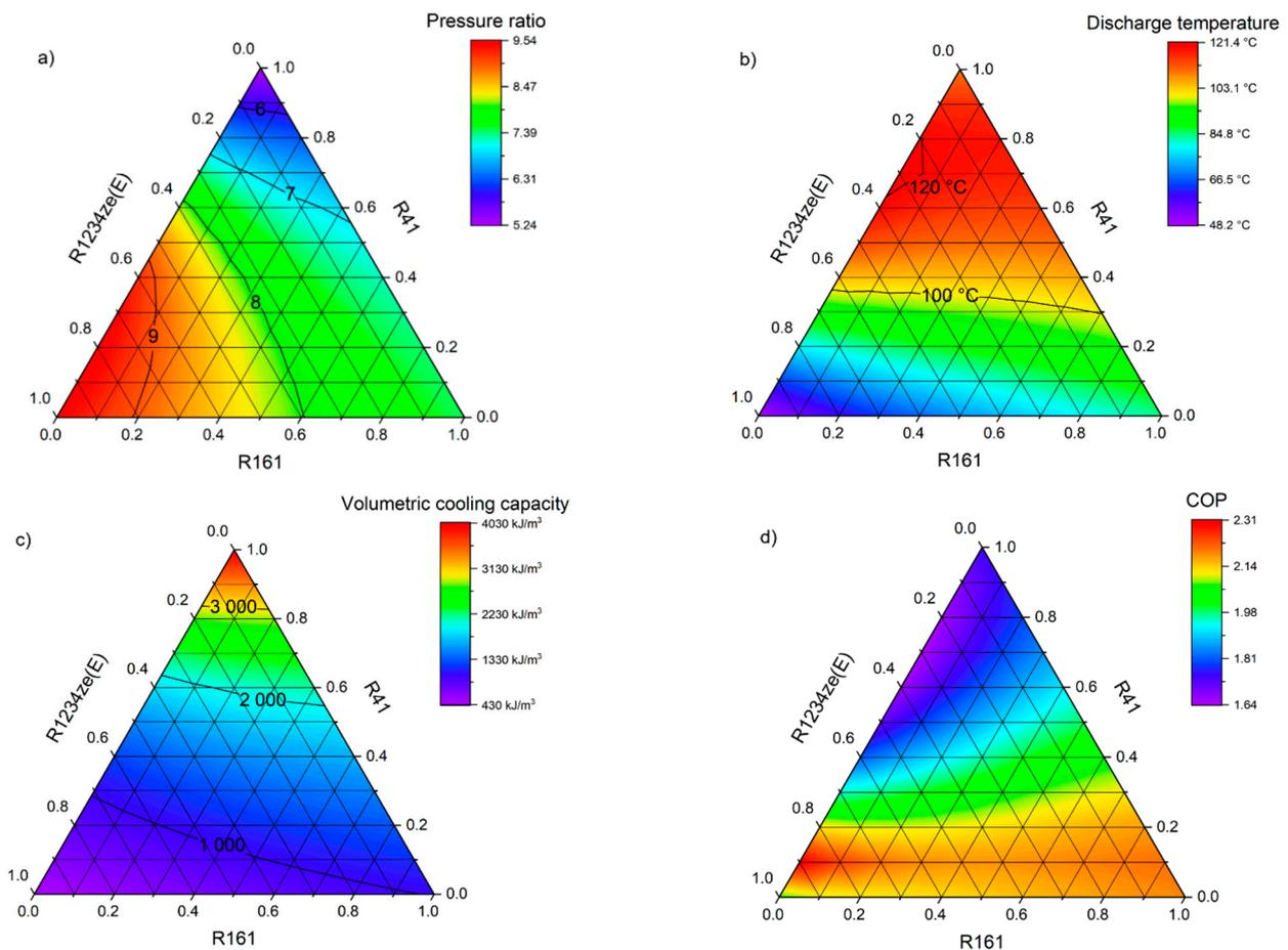
**Figure 10.** Low-temperature system parameters ( $t_e/t_c = -30/30\text{ }^\circ\text{C}$ ) of the R161–R41–R1234ze(E) mixture: (a) pressure ratio; (b) temperature of the refrigerant vapour at the compressor discharge; (c) volumetric cooling capacity; and (d) COP.
