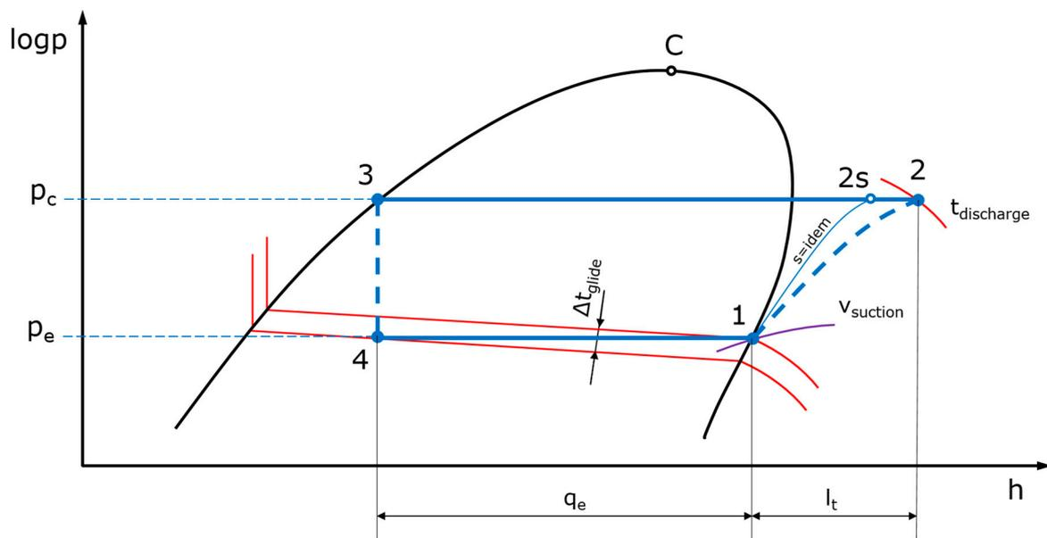
Figure 2. Single stage refrigeration cycle analyzed.
