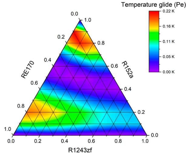
**Figure 15.** Temperature glide at the evaporation pressure for air-conditioning system ( $t_e/t_c = 0/30\text{ °C}$ ) with R1243zf–R152a–RE170 mixture as refrigerant.
