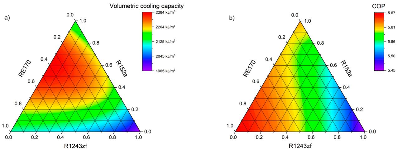
**Figure 16.** Volumetric cooling capacity (a) and (b) the COP for air-conditioning system ( $t_e/t_c = 0/30$  °C) with R1243zf–R152a–RE170 mixture as refrigerant.
