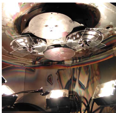
Figure 2. E-beam deposition system: glass substrates mounted on the rotating planetary. The thickness monitor sensor is also visible.
