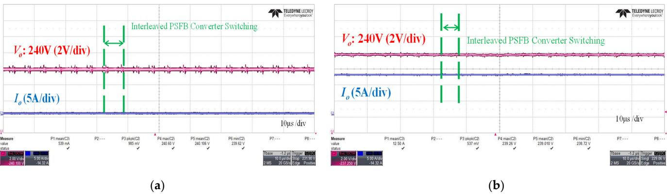
**Figure 16.** Experimental waveforms of the output voltage and output current. (a) At no load. (b) At 3-kW-rated load.
