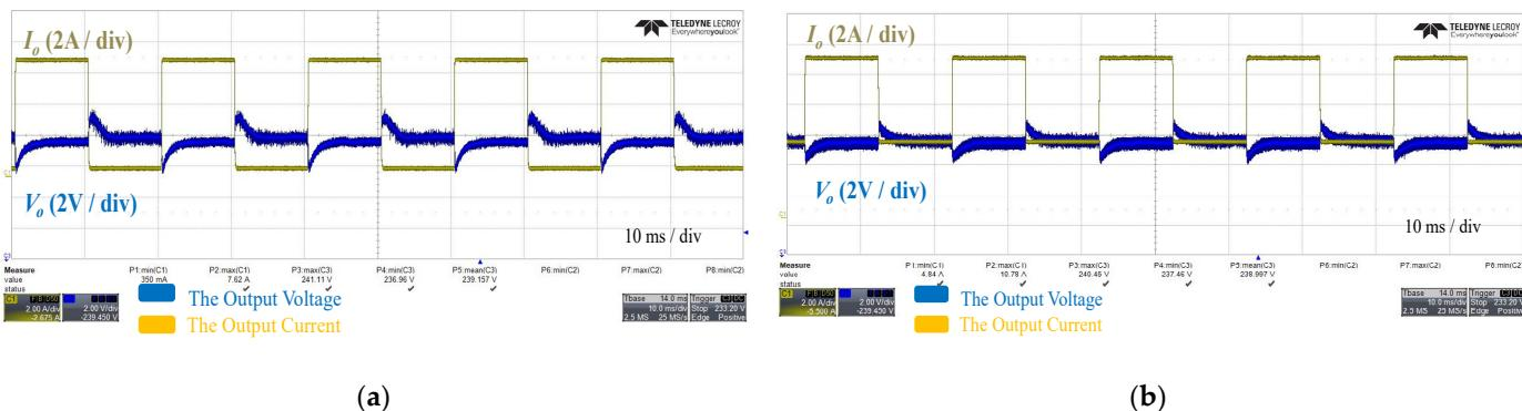
**Figure 21.** Experimental transient waveforms when the dynamic load is performed. (a) From no load to 60% load. (b) From 40% load to full load.
