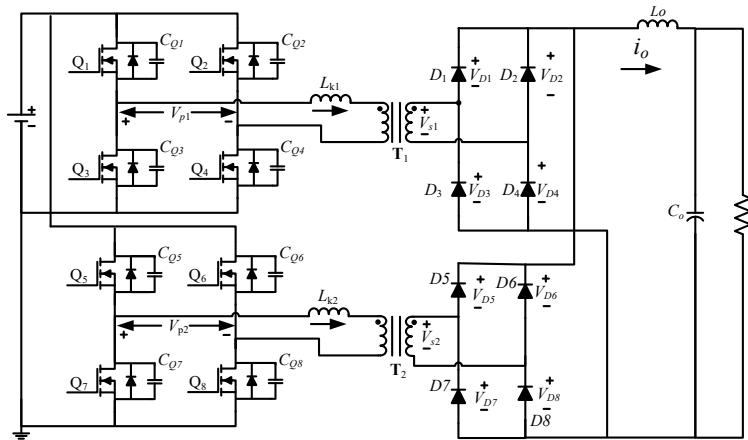
**Figure 2.** Circuit diagram of the proposed phase-shift full-bridge (PSFB) converter.
