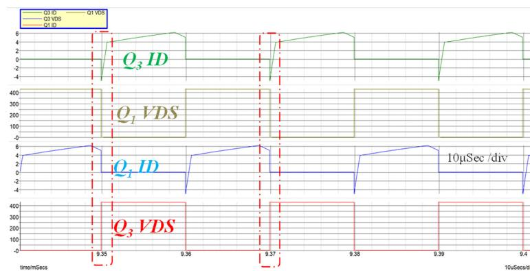
**Figure 13.** Simulated waveforms of the drain current and drain-to-source voltage across the MOSFETs in the same bridge leg.
