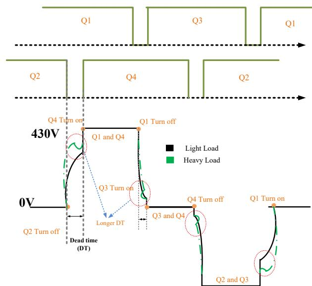
**Figure 6.** Theoretical transformer waveform with a fixed dead time.
