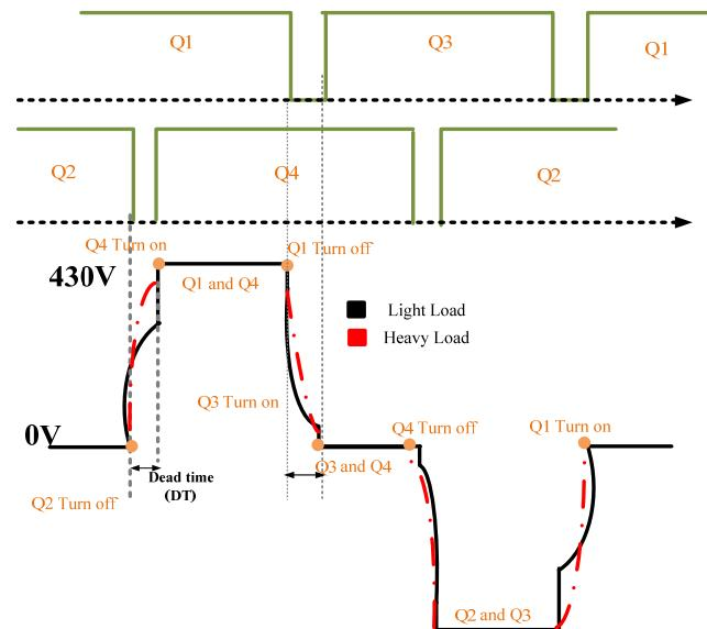
**Figure 7.** Theoretical transformer waveform with dynamic dead time control.
