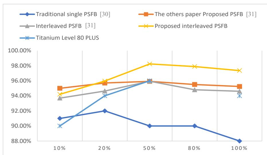
**Figure 22.** Measured conversion efficiency curves.
