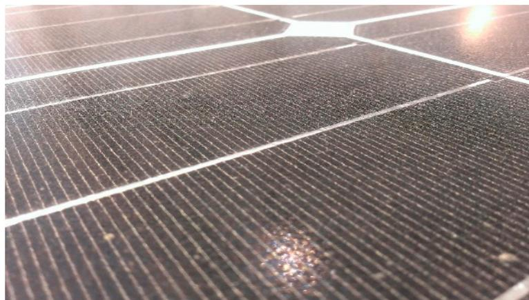
**Figure 17.** The dust settled on the panel surface.
