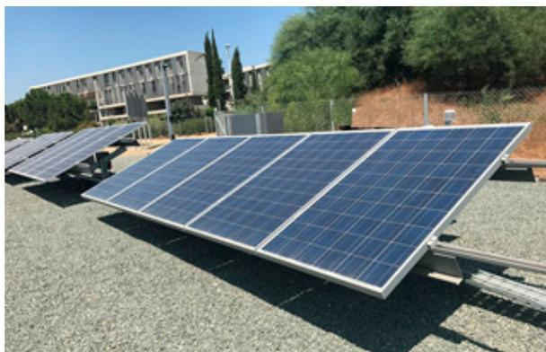
**Figure 2.** Test-bench PV system comprising of a polycrystalline silicon (poly-c Si) photovoltaic (PV) string, sensor network and data acquisition (DAQ) monitoring system, at the FOSS Research Centre in Nicosia, Cyprus.
