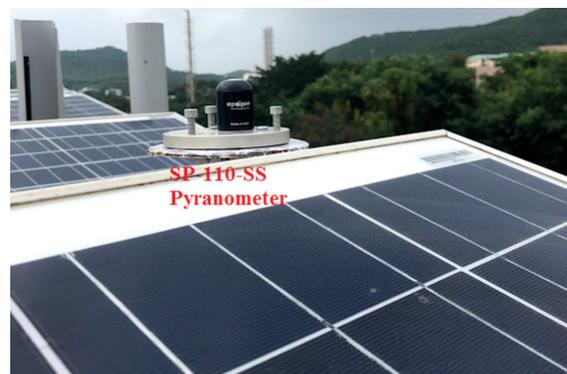
**Figure 3.** Mounted Apogee SP-110-SS pyranometer with alignment of SPV module.
