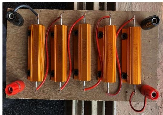
Figure 7. Heat sinkable high wattage resistor.
