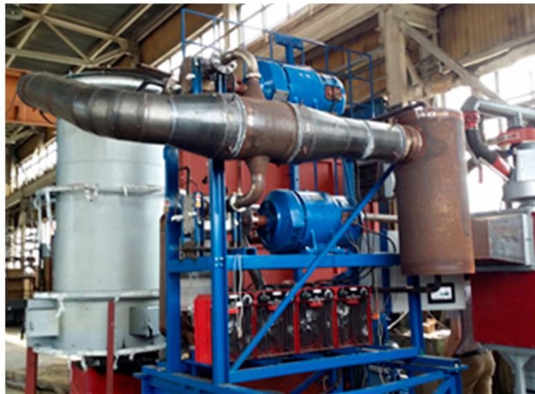
Figure 30. View of a two-stage steam rotary lobe expander with inter-stage superheating [161].
