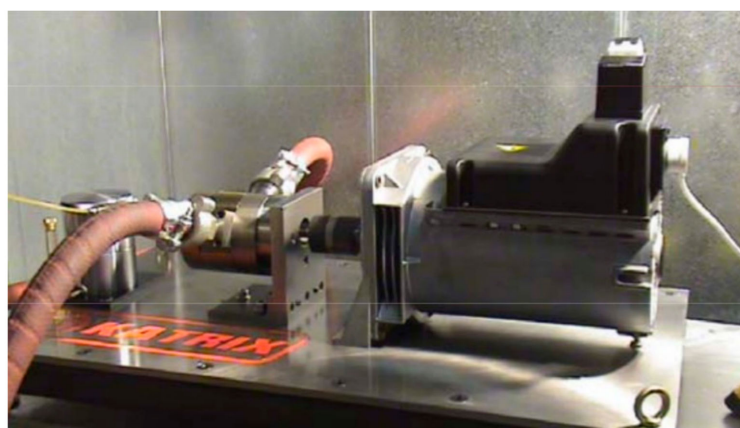
Figure 33. View of a Katrix expander connected to the source of working fluid and generator [162,163].
