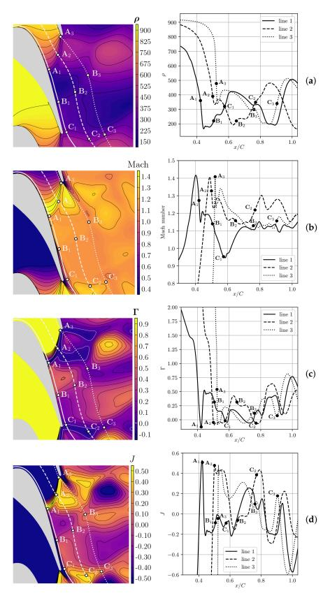
**Figure 7.** Maps of mean quantities (**left**) and their evolution along the three streamlines, labeled 1 to 3 (**right**) for case IC2-LPR: density (row (**a**)), Mach number (row (**b**)),  $\Gamma$  (row (**c**)), and J (row (**d**)).
