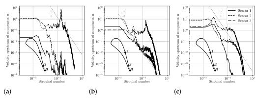
Figure 12. Velocity spectra for cases IC1-LPR (a), IC1-HPR (b), and IC2-LPR (c), evaluated at the three sensor locations shown in the inset.
