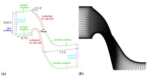
**Figure 2.** Computational domain with boundary conditions (**a**), and close-up view of the grid (**b**), where one point out of four is represented.
