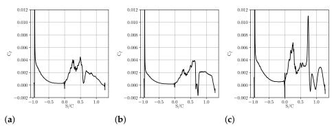
**Figure 6.** Wall distributions of the averaged skin friction coefficient for IC1-LPR (**a**), IC1-HPR (**b**), and IC2-LPR (**c**).
