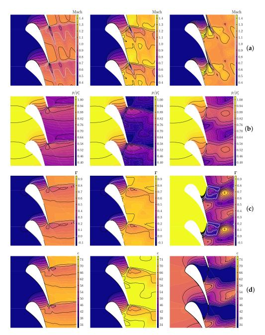
**Figure 4.** Isocontours of averaged quantities: Mach number (row (a)), pressure  $p/p_1^{\circ}$  (row (b)), fundamental derivative  $\Gamma$  (row (c)), and speed of sound (row (d)) for the cases IC1-LPR (left), IC1-HPR (middle), and IC2-LPR (right).
