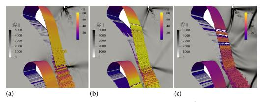
**Figure 3.** Instantaneous iso-surface of the Q-criterion ( $Q = 1000 \text{ s}^{-1}$ ) colored by the velocity magnitude (m/s), replicated three times in the spanwise direction, and snapshot of the relative density gradient in the background for cases IC1-LPR (low pressure ratio) (a), IC1-HPR (high pressure ratio) (b), and IC2-LPR (c).
