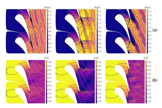
**Figure 8.** Reynolds-averaged Navier–Stokes (RANS) results for the Mach number (a) and normalized pressure  $p/p^{\circ}$  (b). Cases IC1-LPR (**left**), IC1-HPR (**middle**), and IC2-LPR (**right**). For the latter case, the time-averaged unsteady RANS solution is presented.
