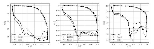
**Figure 9.** Normalized pressure distributions along the wall for cases IC1-LPR (**left**), IC1-HPR (**middle**), and IC2-LPR (**right**).  $\xi/C$  denotes the normalized chordwise coordinate.
