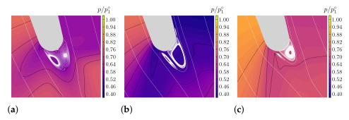
**Figure 5.** Close-up view of the trailing edge: isocontours of average pressure (background) and average stream lines for the cases IC1-LPR (a), IC1-HPR (b), and IC2-LPR (c).
