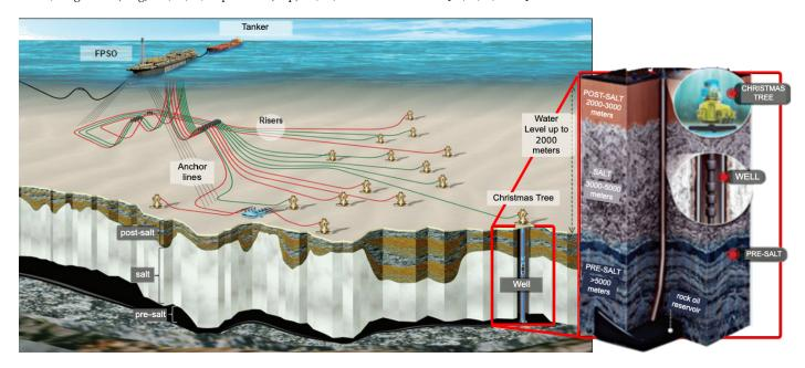
Figure 1. Graphic representation of FPSO and subsea systems.
