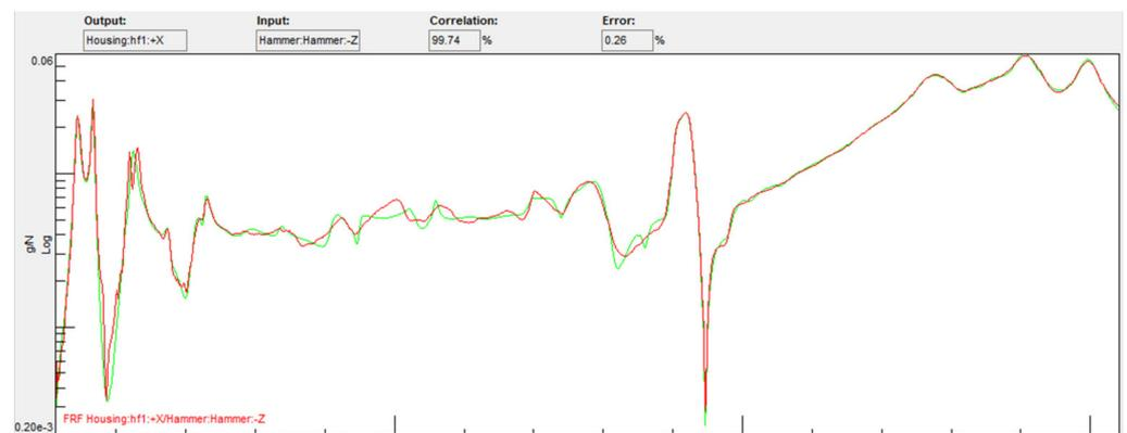
**Figure 9.** Experimental Frequency Response Function vs Curve Fitting for NVH testing.
