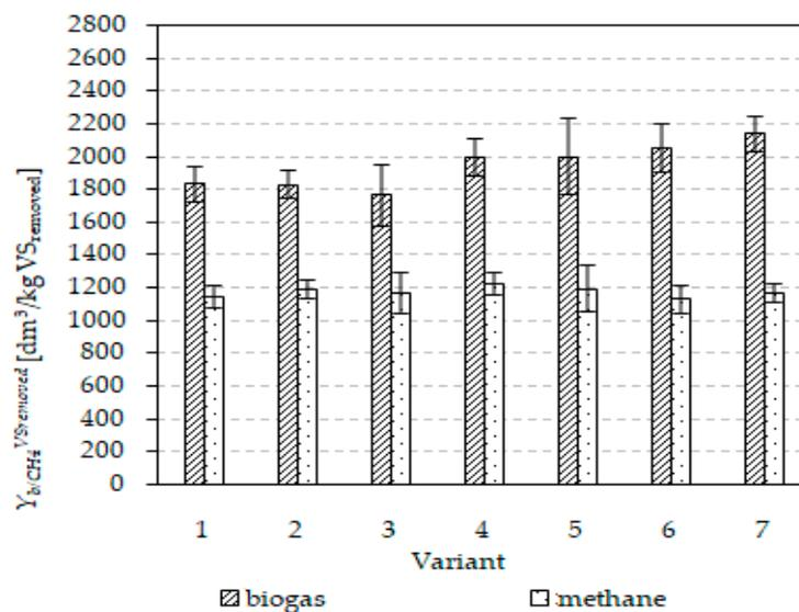
Figure 10. Biogas and CH<sub>4</sub> production in relation to VS removed.
