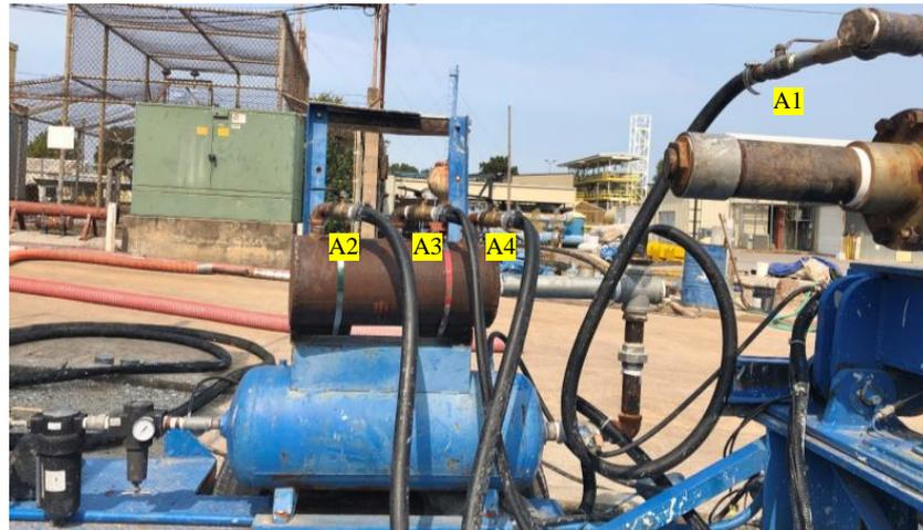
**Figure 2.** Buffer accumulator and air valve. (A1: release the air under static condition; A2, A3, and A4: release the air under countercurrent flow condition).
