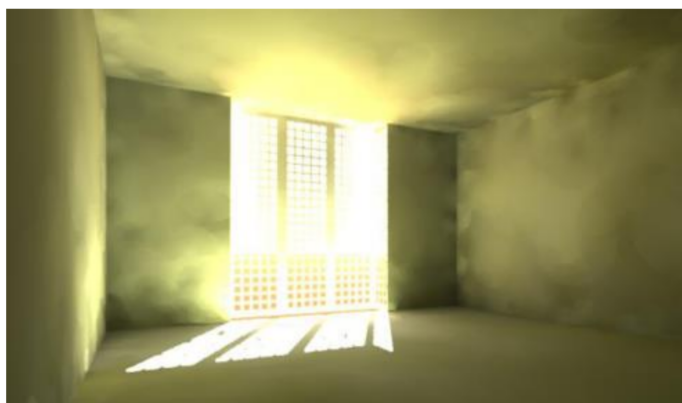
Figure 7. Simulation via Radiance for evaluating lighting level. Reproduced from Batterjee [24].
