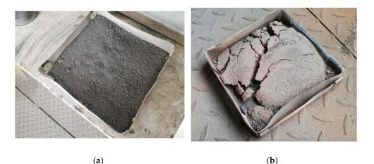
**Figure 13.** Fly ash sample before (**a**) and after decomposition on the grate (**b**).
