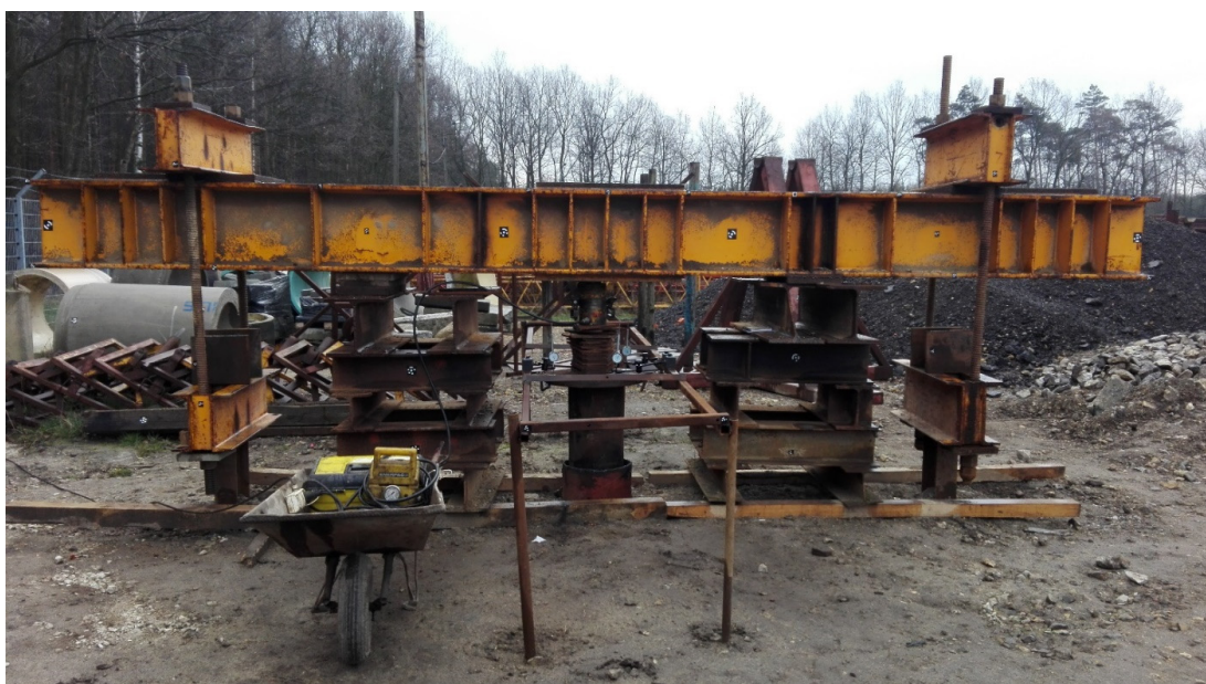
Figure 4. Test stand for traditional static load test and pile bottom capacity test (through inner pipe).
