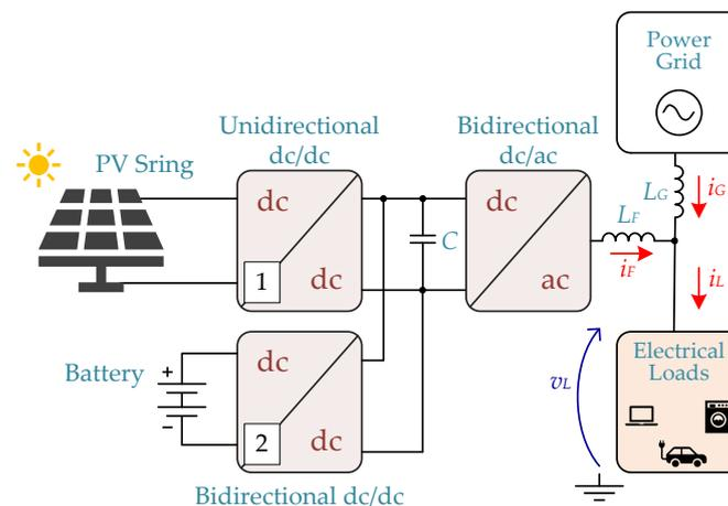
Figure 2. Simplified electrical scheme of a hybrid PV-ESS system.
