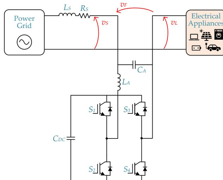
**Figure 22.** Simplified schematic of a transformerless single-phase series APF (TlSeAPF).
