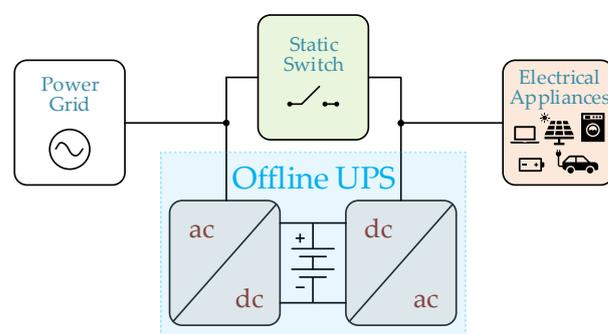
**Figure 26.** Basic structure of an offline UPS.
