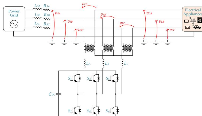
**Figure 18.** Simplified schematic of a three-phase SeAPF based on a voltage source inverter.
