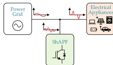
**Figure 12.** Operation principle of a shunt active power filter (ShAPF).
