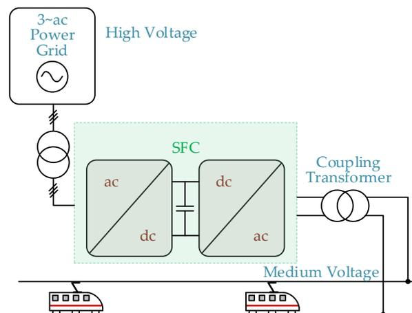
**Figure 32.** Static Frequency Converter (SFC) in electrified railways.
