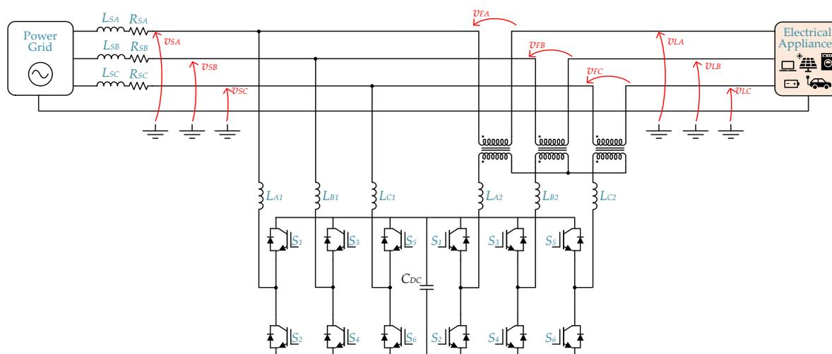
**Figure 19.** Simplified schematic of a three-phase back-to-back power converter to extend the compensation capabilities of the SeAPF.
