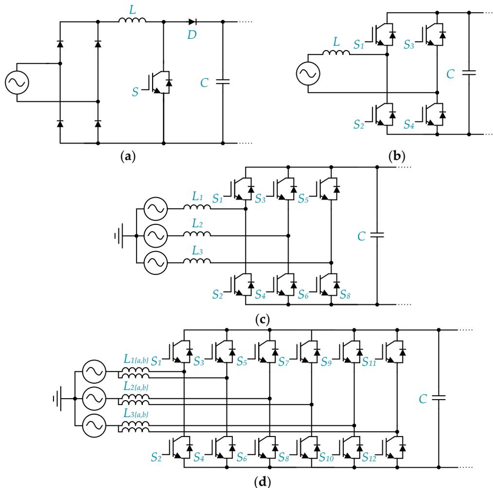
**Figure 9.** Main power electronics topologies applied as front-end power stage of on-board and off-board EV battery charging systems: (a) PFC; (b) Single-phase full-bridge; (c) Three-phase full-bridge; (d) Three-phase full-bridge interleaved.
