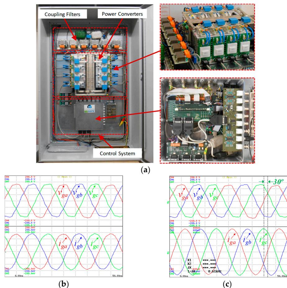
**Figure 11.** Developed off-board EV battery charging system producing reactive power: (a) Example of a laboratory prototype; (b) Experimental results during EV battery charging ( $v_{ga}$ ,  $v_{gb}$ ,  $v_{gc}$ : 50 V/div/ $i_{ga}$ ,  $i_{gb}$ ,  $i_{gc}$ : 10 A/div | 5 ms/div); (c) Experimental results during EV battery charging and producing reactive power ( $v_{ga}$ ,  $v_{gb}$ ,  $v_{gc}$ : 50 V/div/ $i_{ga}$ ,  $i_{gb}$ ,  $i_{gc}$ : 10 A/div | 5 ms/div).
