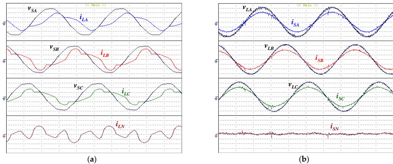
**Figure 25.** Experimental results of a three-phase four-wire UPQC in steady-state operation: (a) Power grid voltages,  $v_{Sx}$ , and load currents,  $i_{Lx}$ ; (b) Load voltages,  $v_{Lx}$ , and power grid currents,  $i_{Sx}$ .
