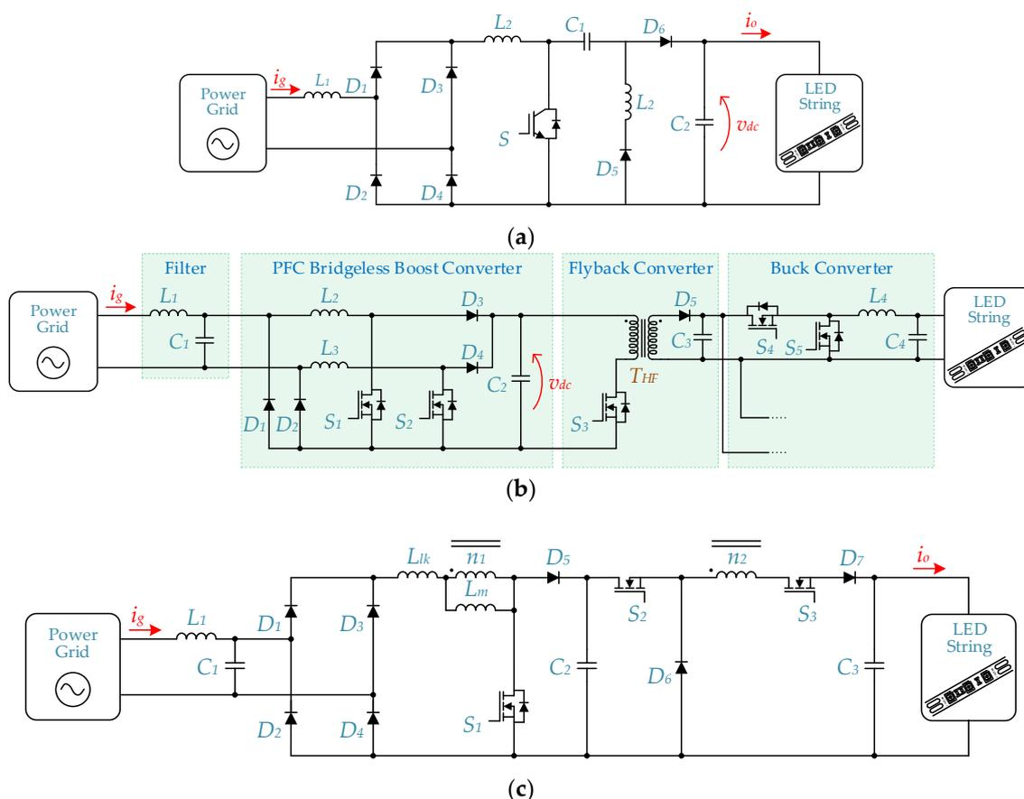
**Figure 37.** LED driver based on: (a) Modified SEPIC converter topology; (b) Flyback converter powered by a PFC bridgeless boost converter; (c) Electrolytic capacitor-less LED driver with coupled inductor based on a PFC boost converter cascaded with a buck converter.
