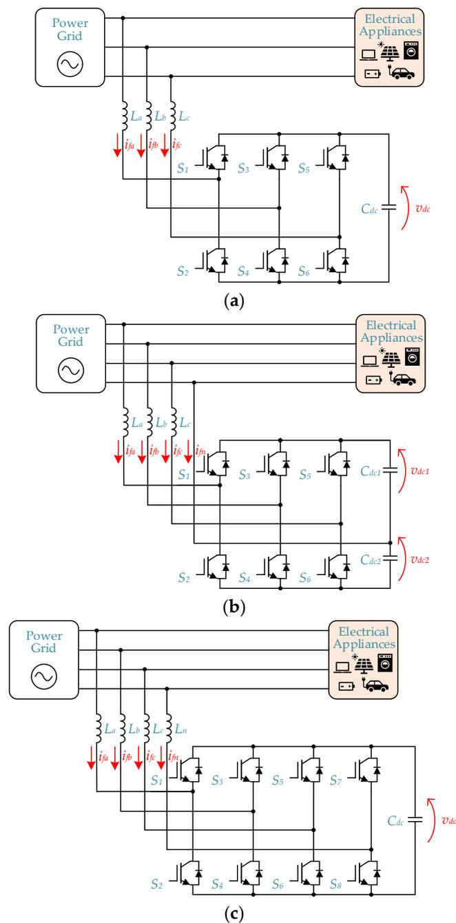
**Figure 14.** Three-phase ShAPFs using ac-dc converters based on: (a) Three-wire three-leg; (b) Four-wire three-leg; (c) Four-wire four-leg.
