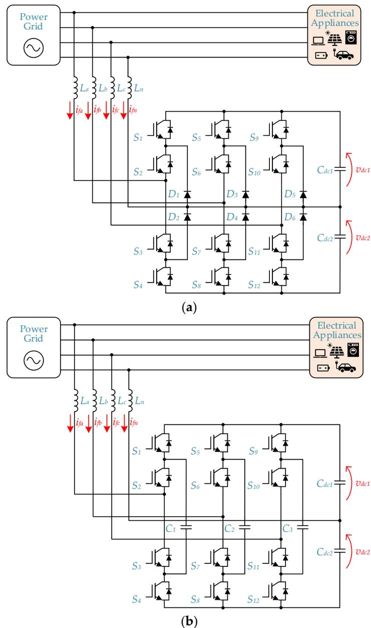
**Figure 16.** Three-phase ShAPF using multilevel ac–dc converters based on: (a) NPC; (b) Flying capacitor.
