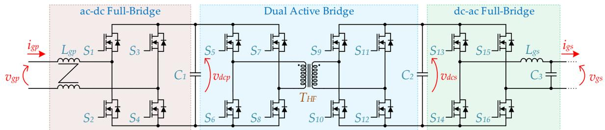
**Figure 5.** Block diagram of the single-phase three-stage SST topology.
