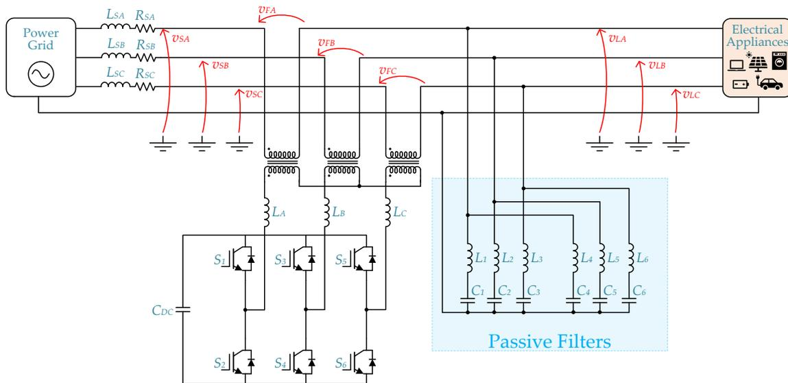
Figure 20. Simplified schematic of a three-phase hybrid series active power filter (HySeAPF).
