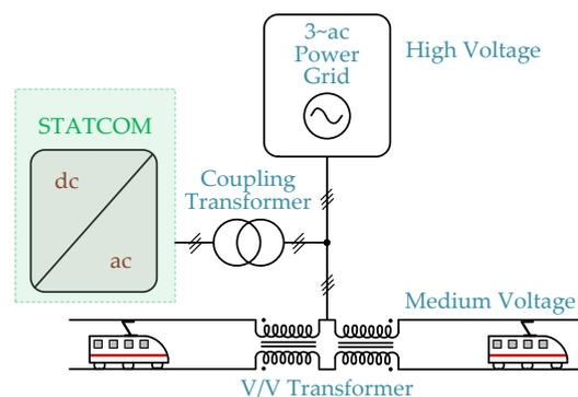
**Figure 31.** Static Synchronous Compensator (STATCOM) in electrified railways.
