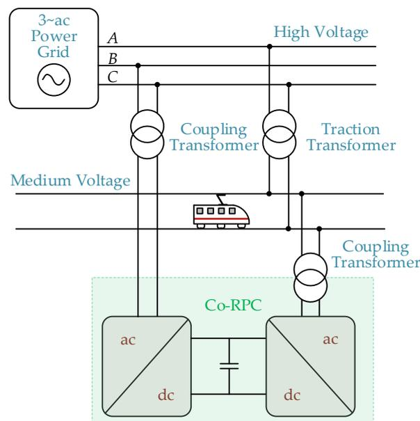
**Figure 34.** Co-phase Rail Power Conditioner (Co-RPC) in electrified railways. A, B, C refer to the three-phase voltages.
