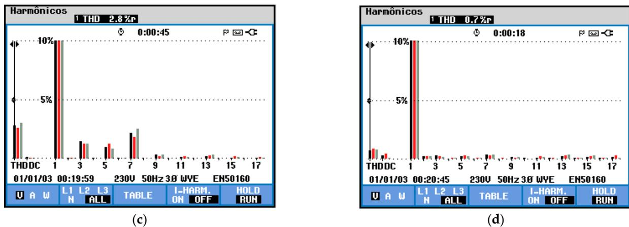
**Figure 21.** Experimental results with a three-phase transformerless series APF (TlSeAPF): (a) Power grid voltages ( $v_{Sa}$ ,  $v_{Sb}$ , and  $v_{Sc}$ ); (b) Load voltages ( $v_{La}$ ,  $v_{Lb}$ , and  $v_{Lc}$ ) and series APF voltages ( $v_{Fa}$ ,  $v_{Fb}$ , and  $v_{Fc}$ ); (c) Harmonic spectrum of the power grid voltages; (d) Harmonic spectrum of the load voltages.
