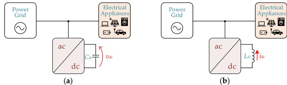
**Figure 13.** Basic structure of a ShAPF based on a: (a) Voltage source converter; (b) Current source converter.
