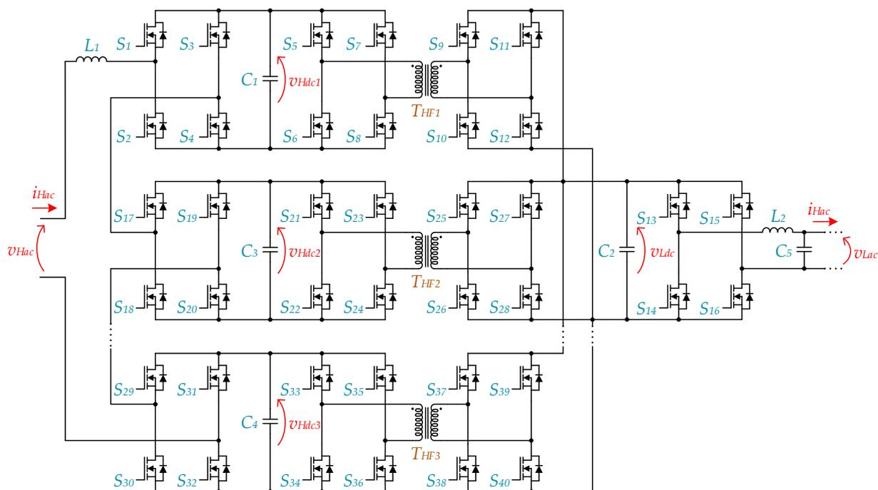
**Figure 6.** Single-phase building block of a three-phase SST topology for wind generation system applications.
