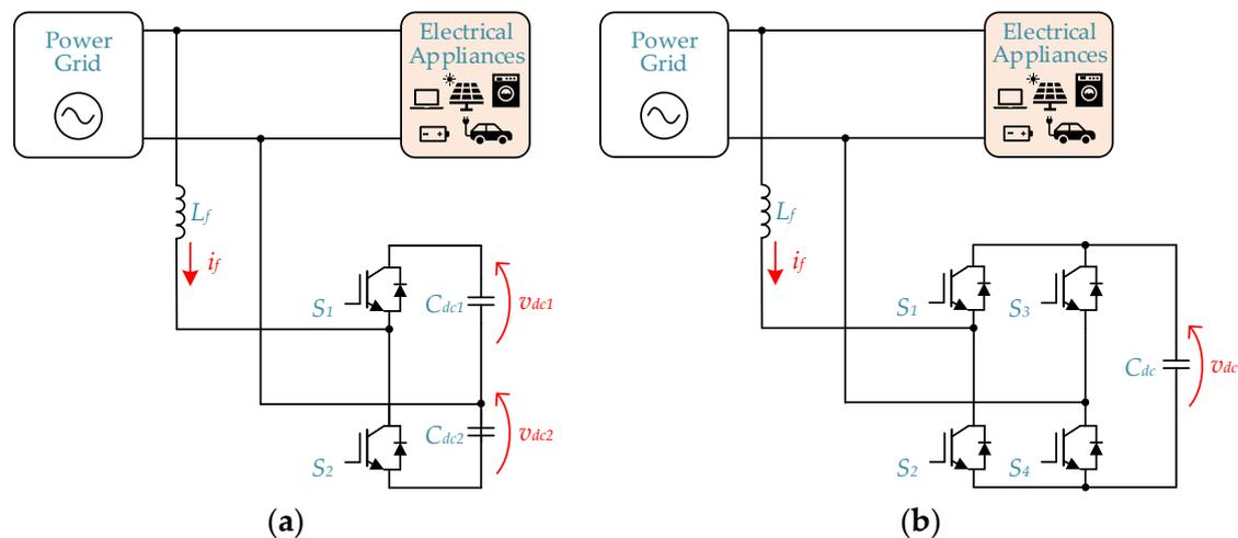
**Figure 15.** Single-phase ShAPFs using ac–dc converters based on: (a) Half-bridge topology; (b) Full-bridge topology.
