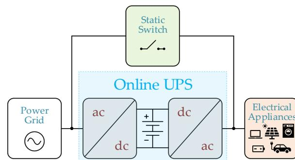
Figure 29. Basic structure of an online UPS.
