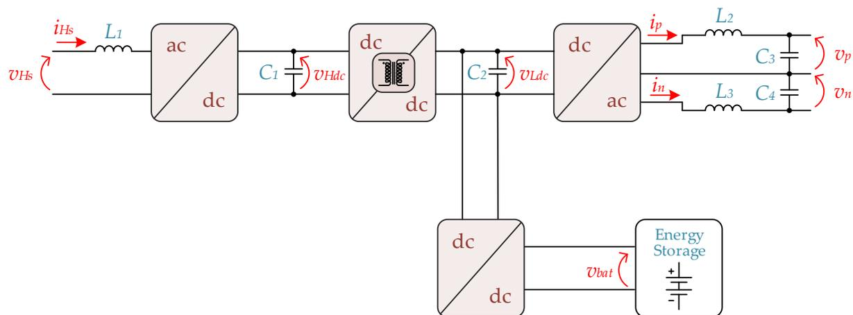
Figure 7. SST applied to energy storage system (ESS).
