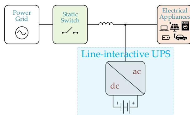
**Figure 27.** Basic structure of the line-interactive UPS with series inductor.
