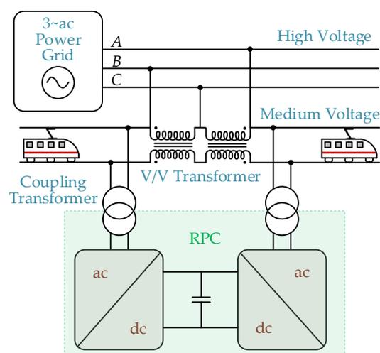
**Figure 33.** Rail Power Conditioner (RPC) in electrified railways. A, B, C refer to the three-phase voltages.
