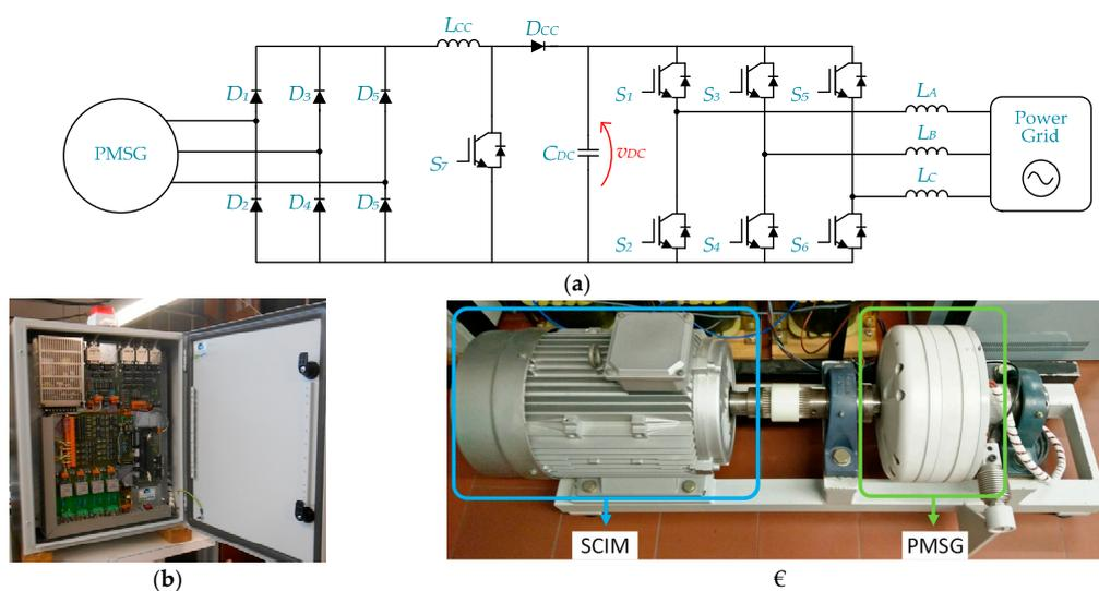
**Figure 3.** Power electronics converter for micro wind turbine: (a) Converter topology; (b) Developed prototype; (c) Laboratory setup to emulate the wind turbine, composed by a squirrel cage induction motor and a permanent magnet synchronous generator.
