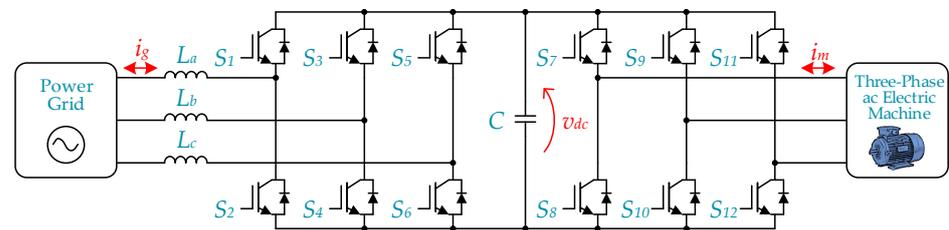
Figure 36. Adjustable speed drive (ASD) with active front-end rectifier.
