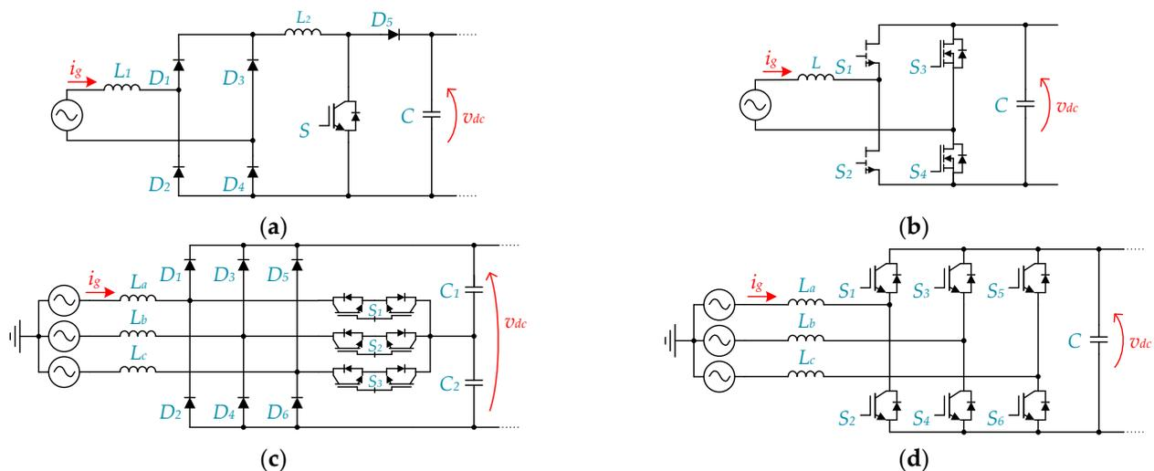
**Figure 35.** Typical PFC converter topologies: (a) Conventional boost PFC converter; (b) GaN totem-pole bridgeless PFC converter; (c) Vienna rectifier; (d) Active front-end.
