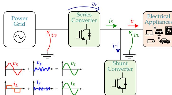
**Figure 23.** Basic principle of both active filters compensating harmonic components.
