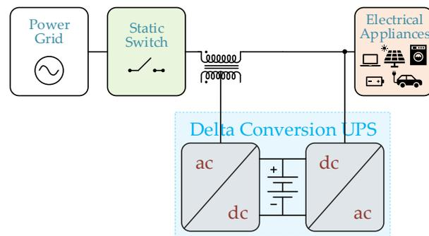
**Figure 28.** Basic structure of the delta conversion line-interactive UPS.
