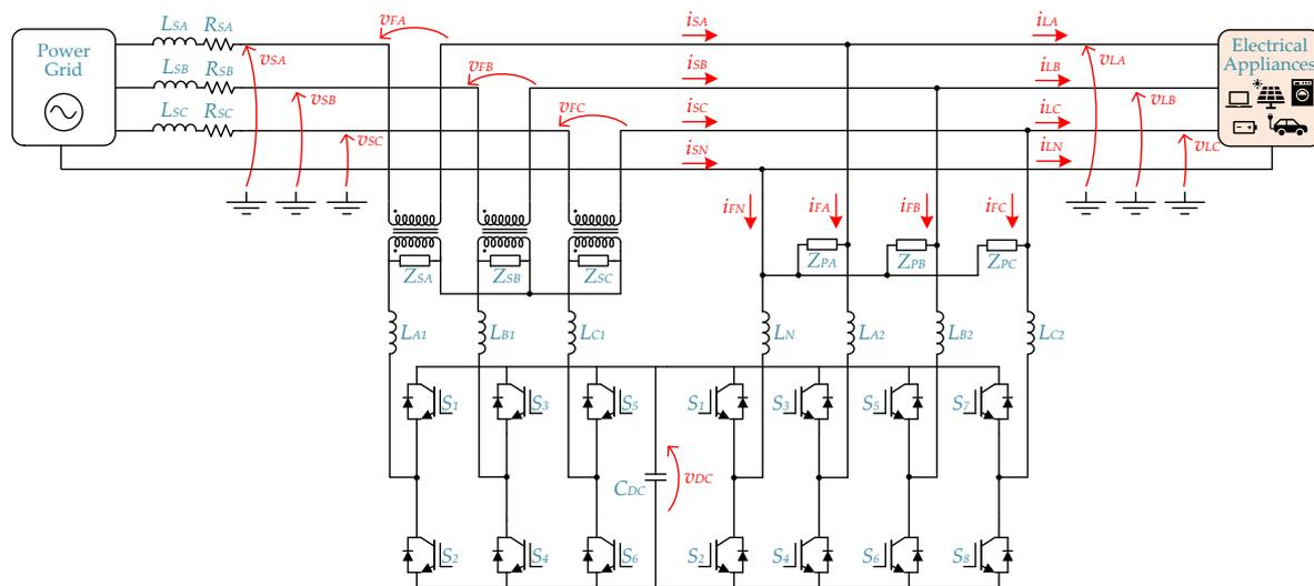
**Figure 24.** Simplified diagram of the UPQC.
