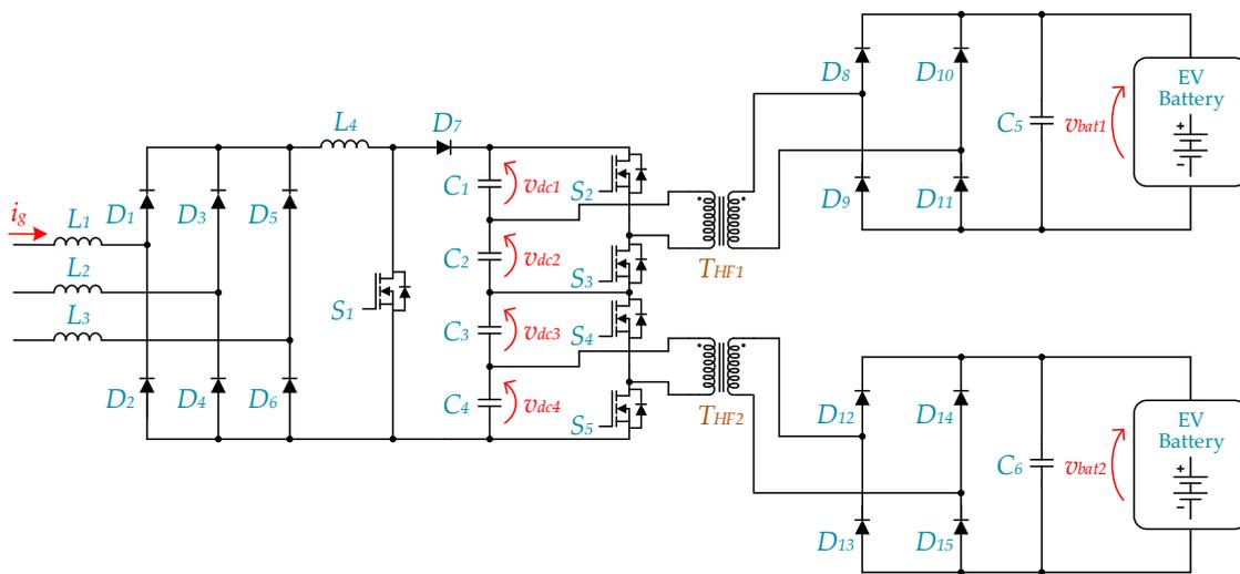
Figure 8. SST for multi-port charging station infrastructure.
