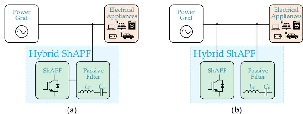
**Figure 17.** Basic structures of hybrid ShAPF using: (a) Series connection; (b) Parallel connection.
