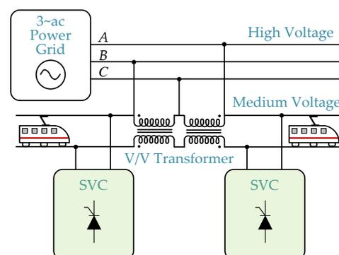
**Figure 30.** Static VAR Compensator (SVC) in electrified railways. A, B, C refer to the three-phase voltages.
