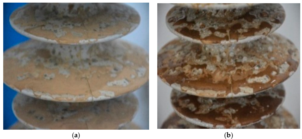
Figure 8. Insulators given fly ash pollutant in (a) dry and (b) wet conditions.
