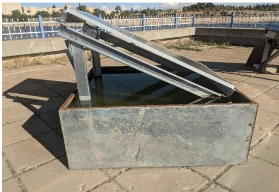
Figure 2. Floating PV panel used in this study.
