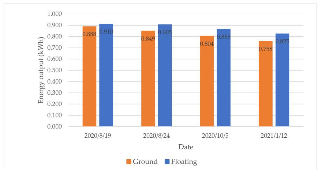
Figure 5. Energy output of different testing days for the period between 10 a.m. and 2 p.m.
