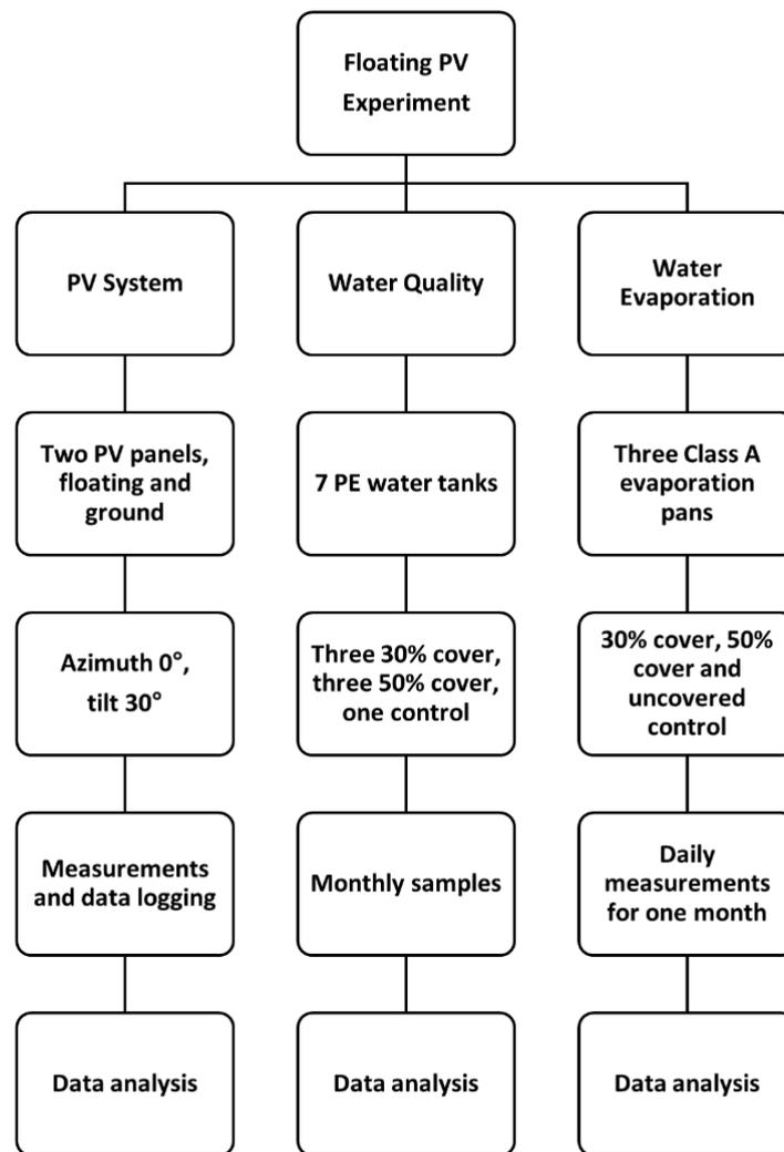
Figure 1. Flowchart of experiment methodology.
