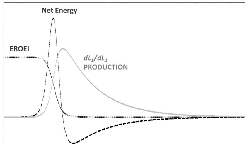
**Figure 5.** Behavior of the  $EROEI_{SCLV}$  and Net Energy according to the SCLV model.
